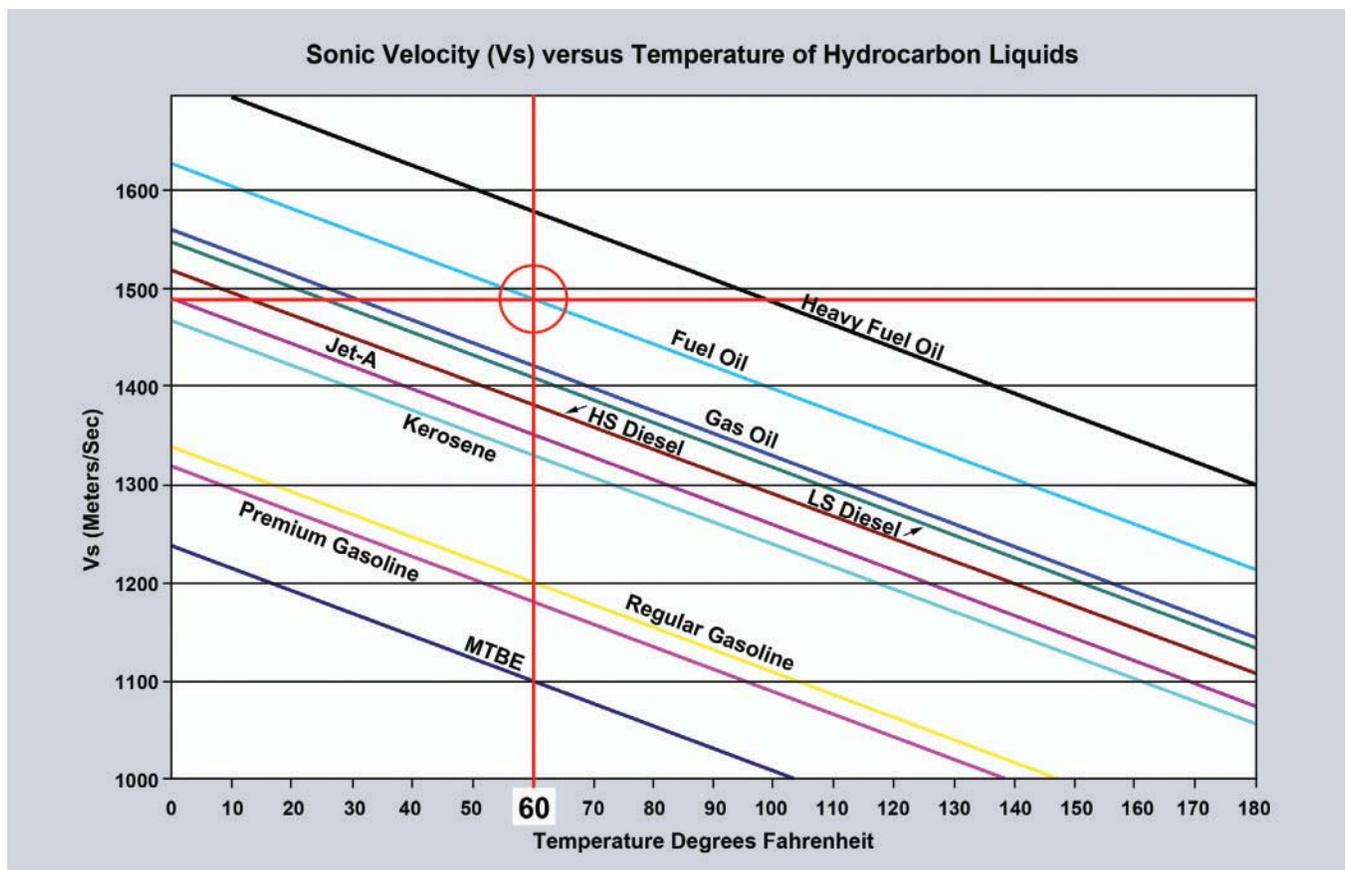
Figure 1. Liquid slope table demonstrating the effect of temperature on the sonic velocity of liquid hydrocarbons.
