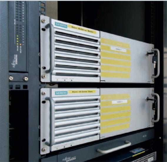
The AS 400 server system of the Simatic PCS 7 process control system collects, processes, and archives the process data
