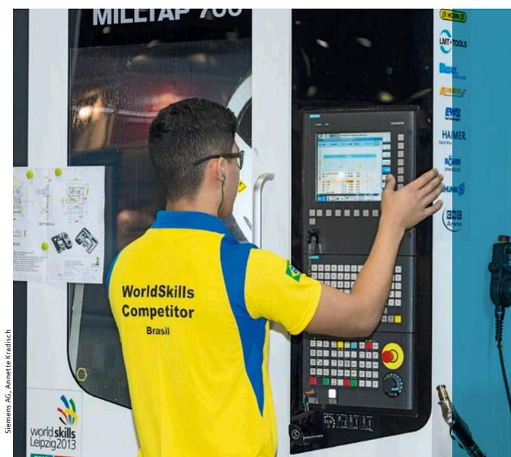
The CNC Sinumerik 840D sl with the Sinumerik Operate user interface makes operation easier for the entrants
