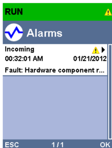
Figure 2: Display of the CPU 1516F-3 PN/DP with alarm text from the system diagnostics
