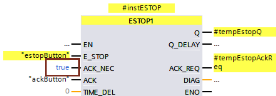
Figure 5-7: "TRUE" and "FALSE" signals as actual parameter
