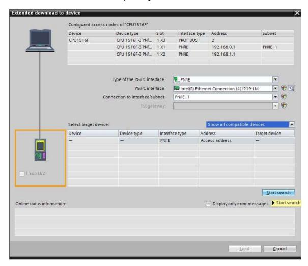
$\rightarrow$  If the controller is shown in the list, it must be selected before the download can be started. ( $\rightarrow$  CPU1516F-3 PN/DP  $\rightarrow$  Load)
