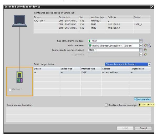
→ If the controller is shown in the list of target devices, it must be selected before starting the download. (→ CPU1516F-3 PN/DP → Load)
