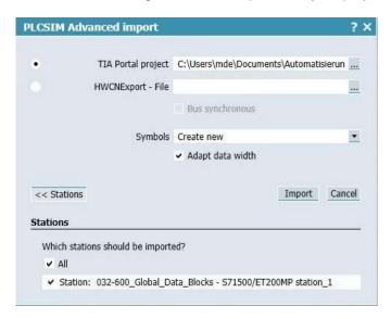
→ Double-click the coupling for the created station "S7-1500-ET 200MP station\_1" to open it. The inputs and outputs from the tag table of the S7-1500 station are now available for further use in the simulation. Select "Save all". (→ S7-1500-ET 200MP station 1 → III)
