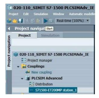
→ When the simulation is started, PLCSIM Advanced is also automatically activated in the background. This allows you to test the access to the inputs and outputs of the S7-1500 station in SIMIT. Clicking on " again ends the simulation in SIMIT. (→ )
