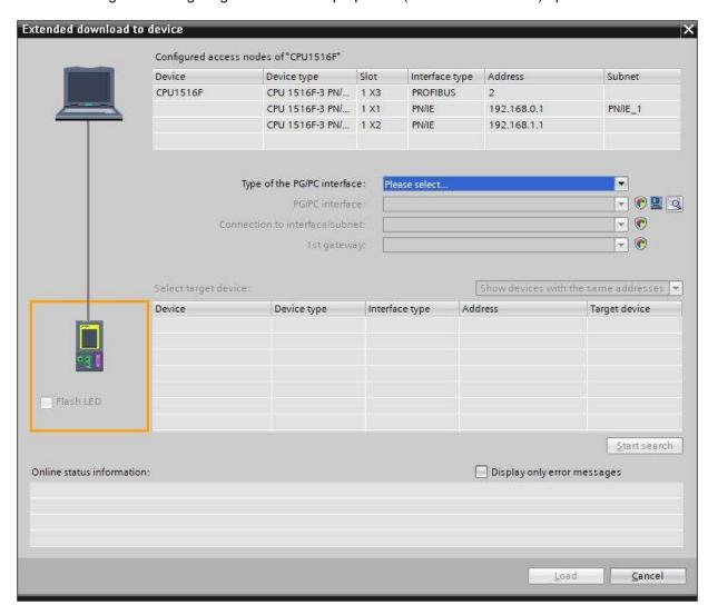
$\rightarrow$  First, the interface must be correctly selected. This happens in three steps.  $\rightarrow$  Type of the PG/PC interface  $\rightarrow$  PN/IE
