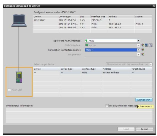
$\rightarrow$  If the controller is shown in the list of target devices, it must be selected before the download. ( $\rightarrow$  CPU1516F  $\rightarrow$  Load)
