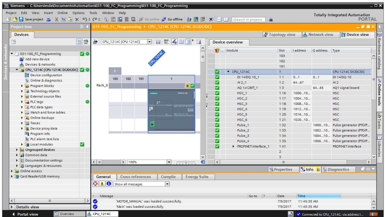
Figure 1: Online view of device configuration
