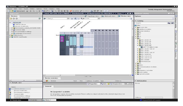
12. We drag the output module '4DO x DC24V / 0.5A HF' to slots 5 and 6. ( $\rightarrow$  DO  $\rightarrow$  4DO x DC24V / 0.5A HF  $\rightarrow$  6ES7 132-4BD00-0AB0)
