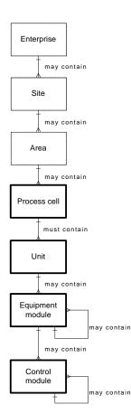
If, when structuring the plant, the physical model according to DIN EN 61512-1 is used (refer to Figure 3) which is largely identical to the U.S. standard ISA-S88.01-1995, *PCS* 7 enables the setup of a type-defined hierarchy.
