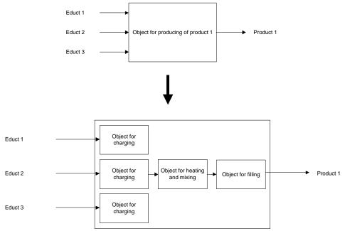
Figure 2: Function of the reactor and its sub-functions
