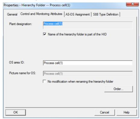
8. In the subheading 'AS-OS Assignment' a hierarchy folder is assigned to an automation system (AS) and to an operator system (OS). In our project, two ASs (AS1 = CPU 414-3 DP and AS2 = AS RTX Box) and one OS are available for selection. The system enters the latter automatically. We select AS1 as the AS. All properties are accepted with OK.
