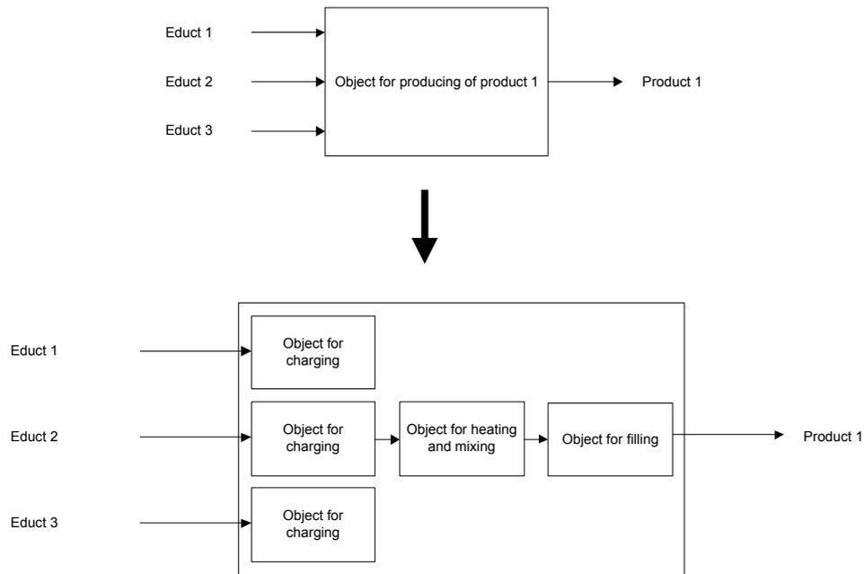
Figure 2: Function and subfunctions of the reactor
