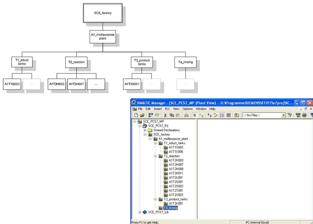
Figure 1: From physical model to plant hierarchy
