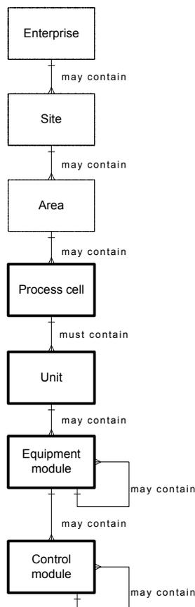
If when structuring the plant the physical model according to DIN EN 61512-1 (refer to Figure 3) is used -which is largely identical with the American standard ISA-S88.01-1995- the **PCS7** provides the option of setting up a type-defined hierarchy.
