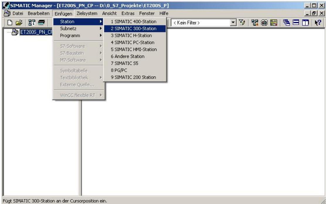
6. With a double click, open the configuration tool for the '**Hardware**' (→ Hardware)
