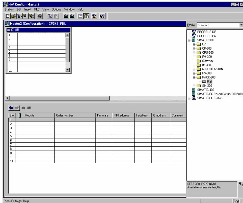
After the insert, a configurations table for the configuration of the Rack 0 appears automatically.
