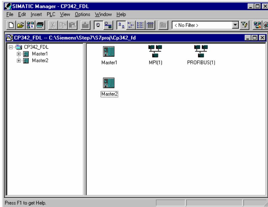
19. Open the configuration tool for the **Hardware** with a double click (→ Hardware).
