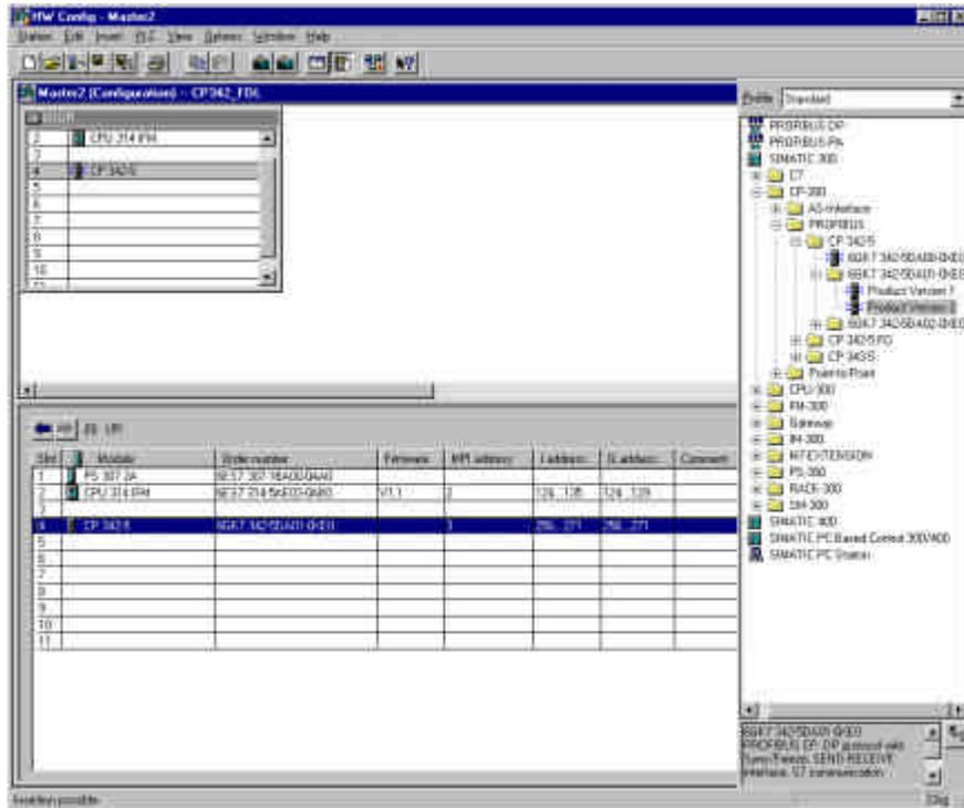
26. **Set the Operation Mode to DP master** and accept with **OK** ( → Operation Mode → DP master → OK).
