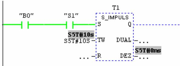
6.3. The signal chart and signal state can be monitored in a FBD.
