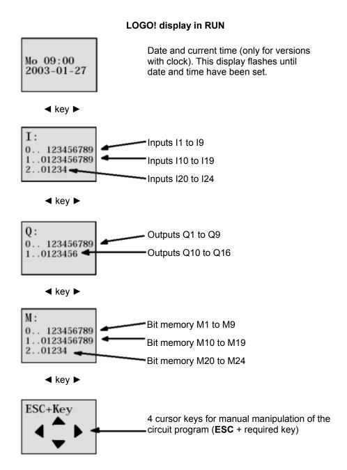
LOGO! processes the program in RUN. To do so, LOGO! starts by reading the states of the inputs, determines the states of the outputs based on the program you have specified and switches the relays at the outputs on or off.
