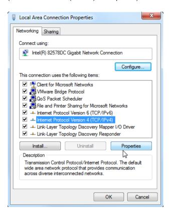
You can then set the 'IP address' and the 'Subnet mask' and apply with 'OK'.
