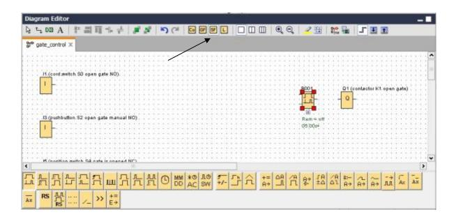
Place the remaining blocks B002 to B016 and set the times for B007 and B016.
