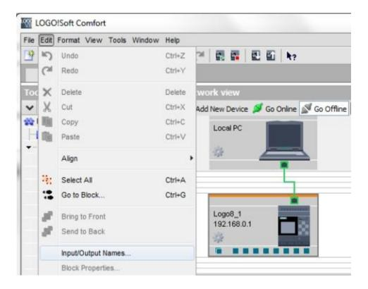
Enter the I/O names of the plant gate control and close the window with **OK**.
