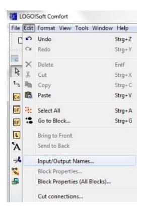
Here you can assign connector names (symbol assignment) to the **input terminals and output terminals** to get a better overview.
