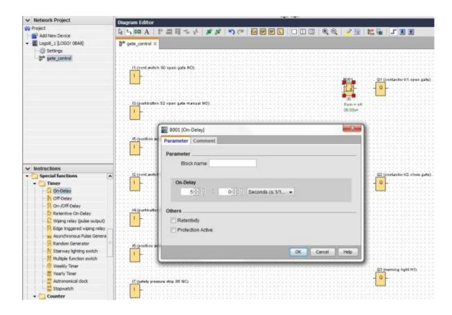
The block functions can be displayed in the programming interface using buttons.
