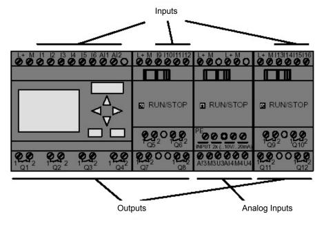
The inputs are specified with the letter I and a number. When you look at LOGO! from the front, you can see the connectors for the inputs at the top. Only with analog modules LOGO! AM2 and AM2 PT100 are the analog inputs on the bottom. The outputs are specified with the letter Q and a number. The connectors of the outputs can be seen at the bottom in the figure.
