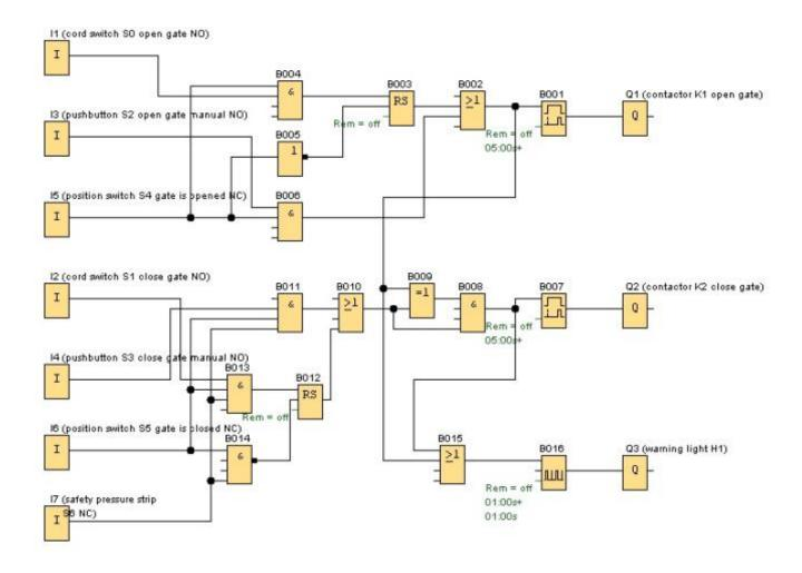
The cord switch **"OPEN GATE"** or **"CLOSE GATE"** initiates the movement of the gate if the opposite direction is not switched on. The travel ends when the respective limit switch is reached. The closing process is also interrupted by the safety pressure strip.
