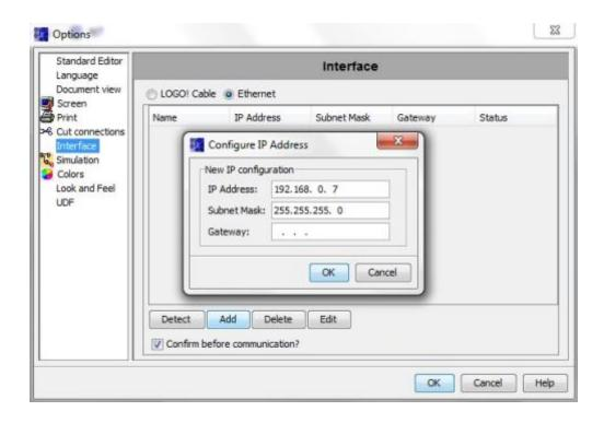
To test the settings, connect the LOGO! with the PC using the network cable and click **Detect**.
