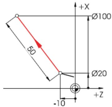
Specification of the end point in Z and an angle
