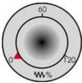
Due to the fact that the machining plan has not yet been executed with control, turn the feedrate potentiometer to zero position to ensure that you keep everything under control from the beginning.
