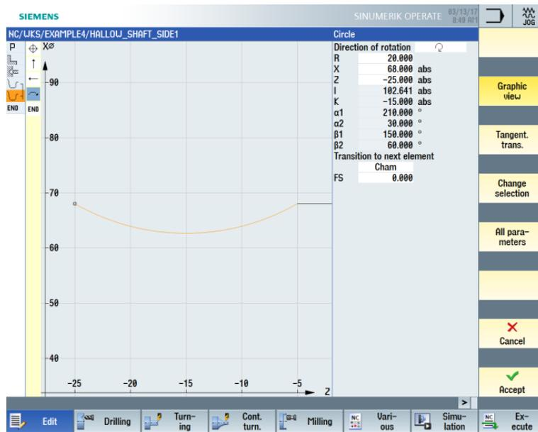
Figure 9-15 Entering the arc for the contour
