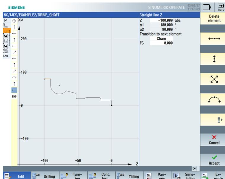
Geometry and technology constitute a unit in programming. The subsequent technological machining operations are applied to the contour.
