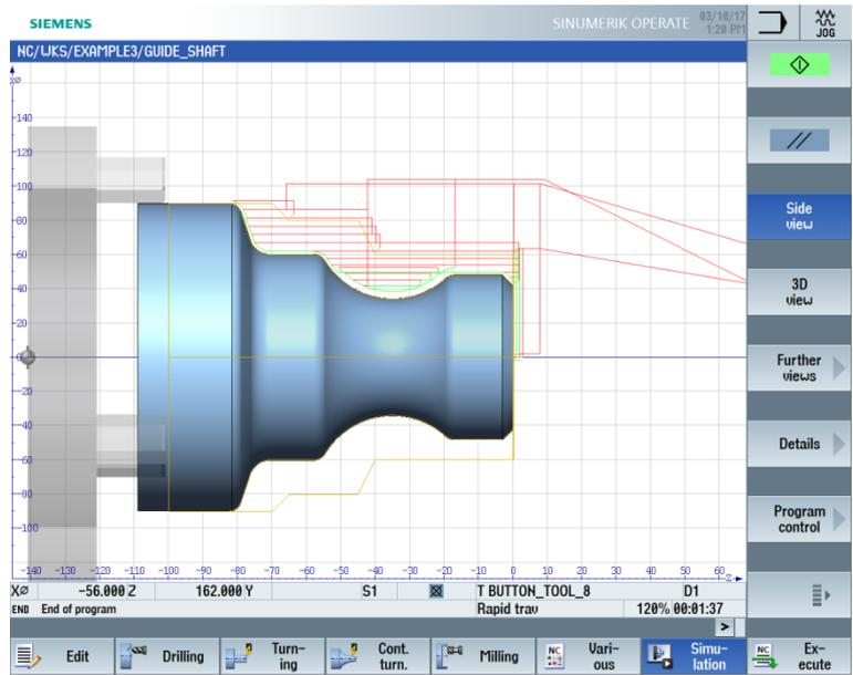
Figure 8-26 Residual stock removal simulation
