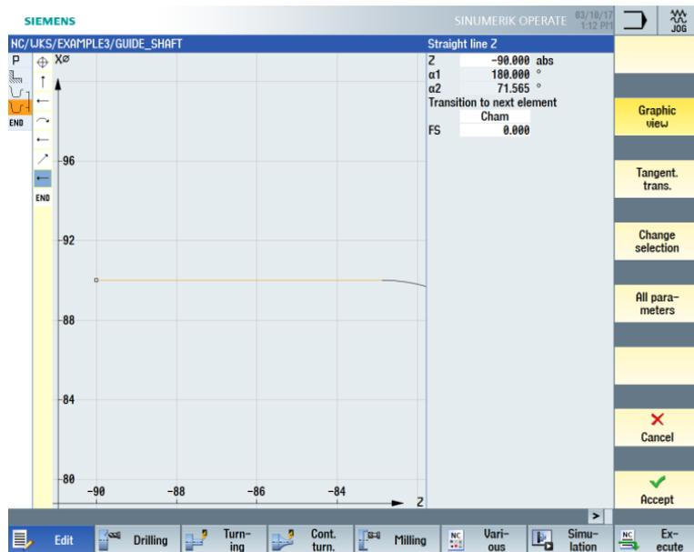
Figure 8-19 Entering the horizontal straight-line segment for the contour
