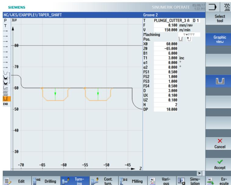
Figure 6-47 Grooves – Graphic view
