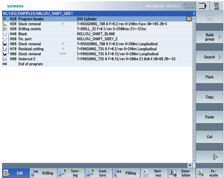
Figure 9-27 Machining plan with undercut
