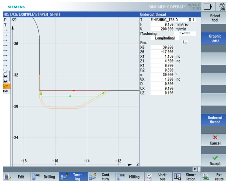
Figure 6-40 Thread undercut – Graphic view
