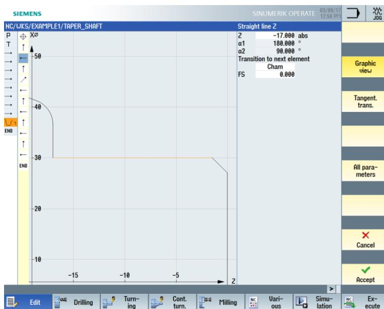
Figure 6-22 Entering the horizontal straight-line segment for the contour
