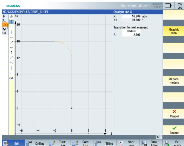
Figure 7-8 Entering the vertical straight-line segment for the contour
