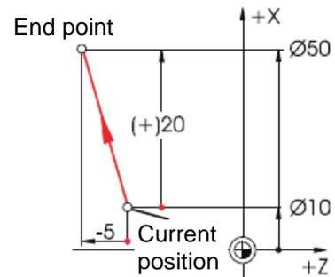
With incremental specifications, the difference values between the current position and the end point must always be entered while taking the direction into account.
