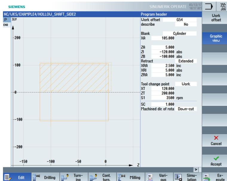
Figure 9-43 Workpiece dimensions in the program header
