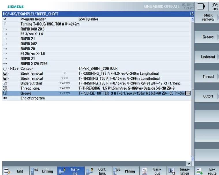
Figure 6-49 Machining plan with grooves
