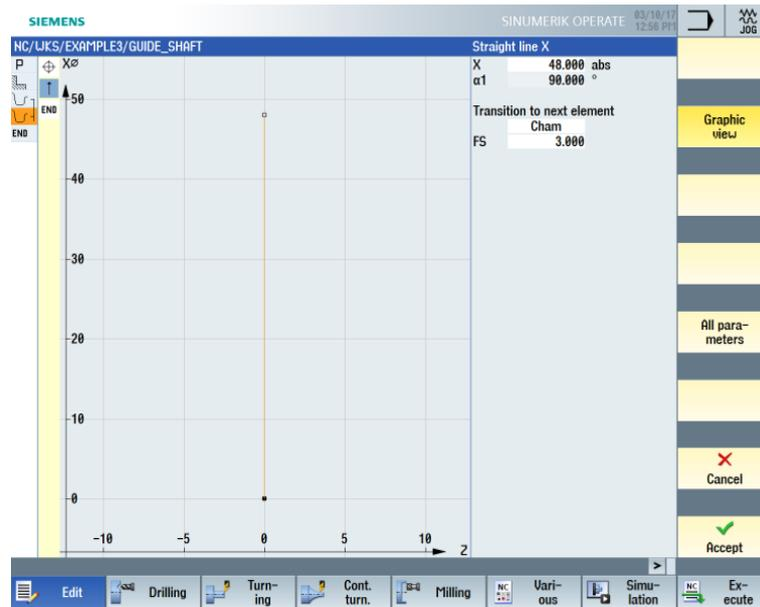
Figure 8-9 Entering the vertical straight-line segment for the contour
