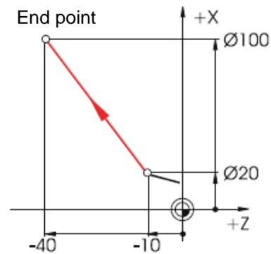
With absolute specifications, the absolute coordinate values of the end point must always be entered (the current position is not considered).
