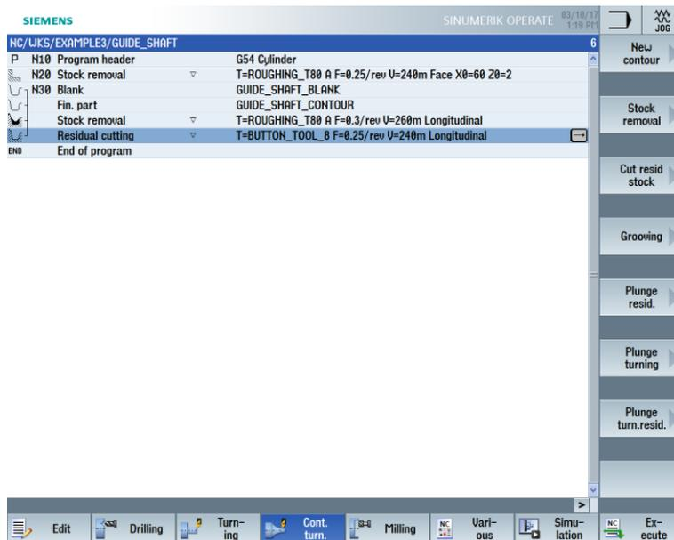
Figure 8-25 Machining plan with residual stock removal
