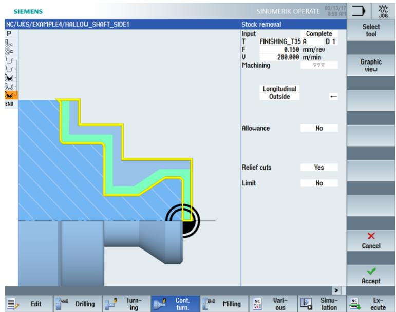
Figure 9-23 Finishing the contour
