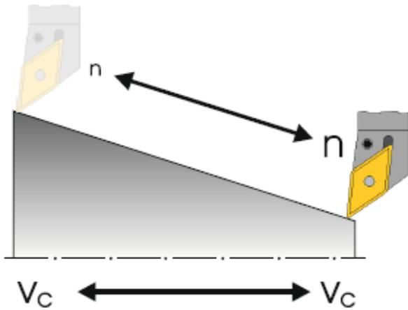
To ensure that the selected cutting rate is the same at every workpiece diameter, the speed is adjusted by the controller with command G96 = Constant cutting rate. This is carried out by DC motors or frequency-controlled three-phase motors. As the diameter decreases, the speed increases theoretically to infinity. To avoid danger due to excessive centrifugal forces, a speed limitation of  $n = 3000$  rpm for example, must be programmed. In DIN format, the block would have the following form:
