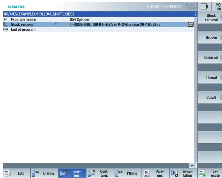
Figure 9-45 Machining plan after face turning
