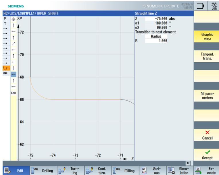
Figure 6-29 Entering the horizontal straight-line segment for the contour
