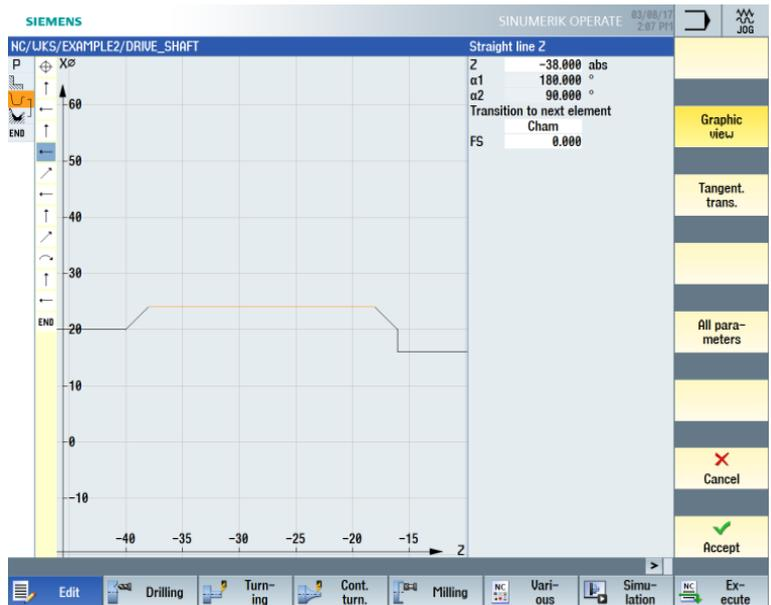
Figure 7-11 Entering the horizontal straight-line segment for the contour
