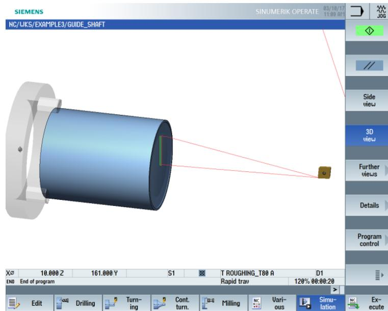
Figure 8-4 Face turning simulation
