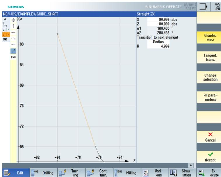
Figure 8-18 Entering the inclined straight-line segment for the contour
