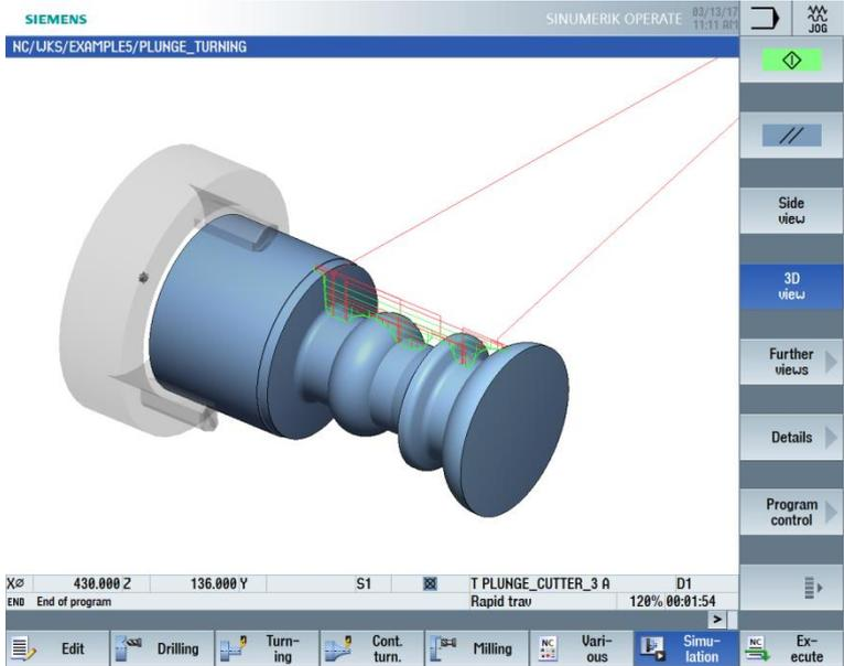
Figure 10-9 Simulation – 3D view (with display of the traversing paths)
