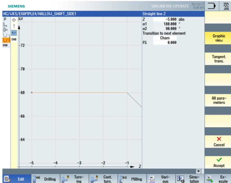
Figure 9-14 Entering the horizontal straight-line segment for the contour
