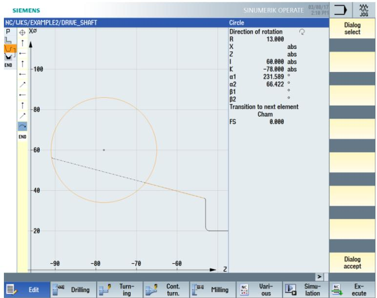
Figure 7-17 Confirming the contour selection
