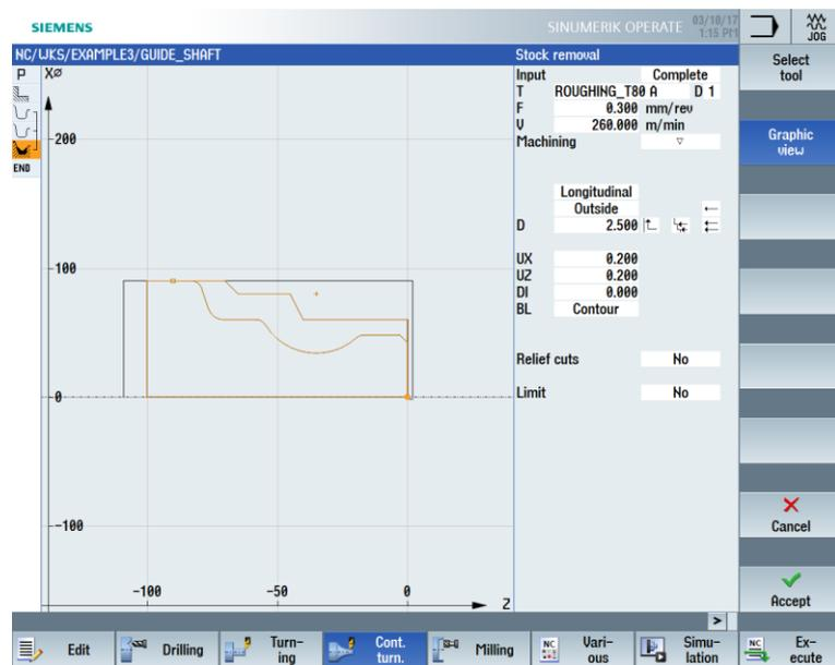
Figure 8-21 Removing stock from the contour
