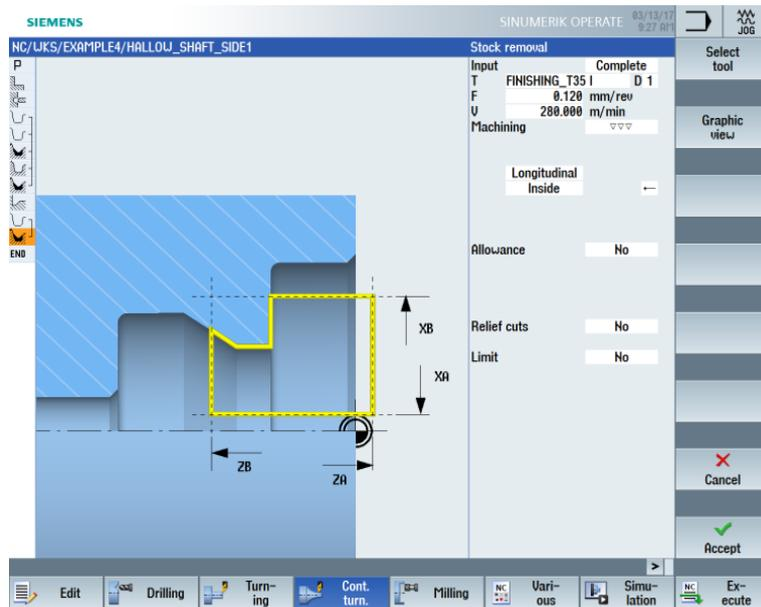
Figure 9-35 Finishing the contour
