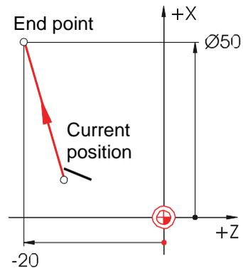
With absolute specifications, the absolute coordinate values of the end point must always be entered (the current position is not considered).
