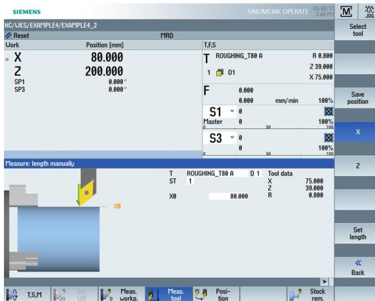
Figure 5-10 Tool measurement – Setting length X
