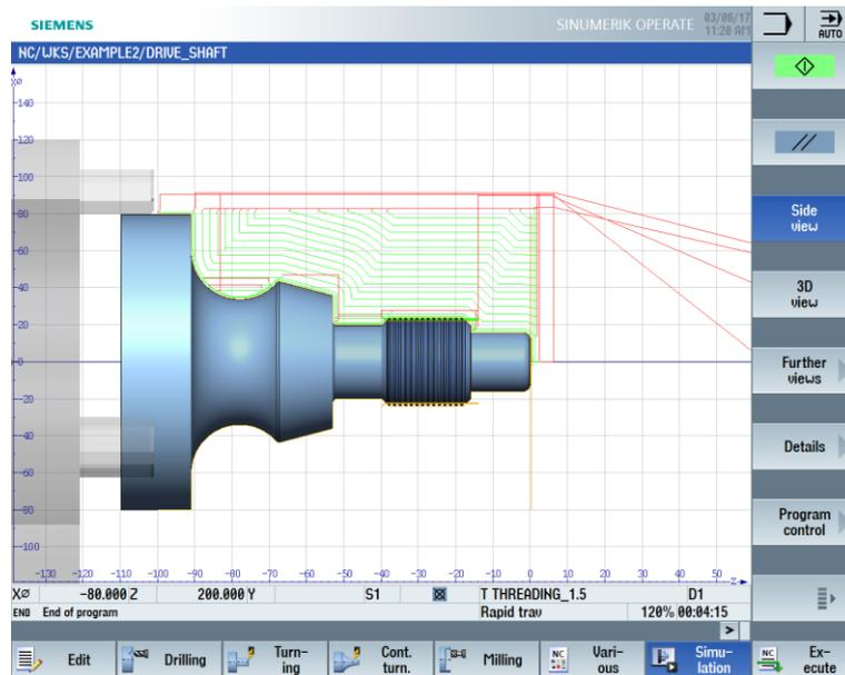
Figure 3-8 Side view (display tool path, activated)
