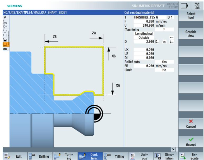
Figure 9-22 Stock removal of residual material from contour
