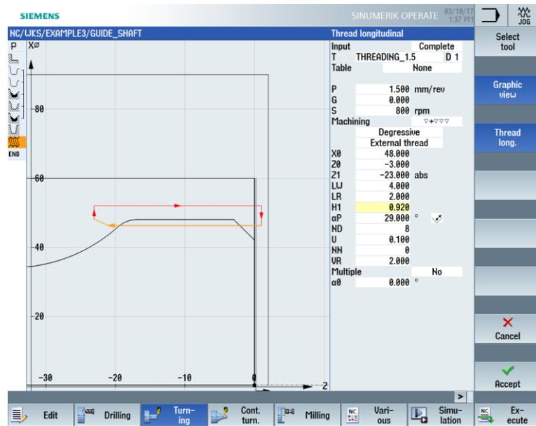
Figure 8-33 Producing the thread
