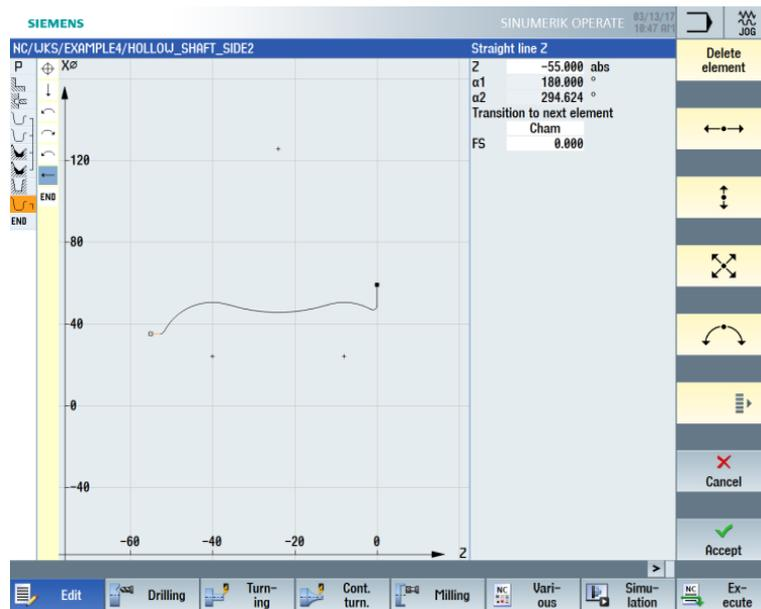
Figure 9-61 Finished part contour of the second side, internal
