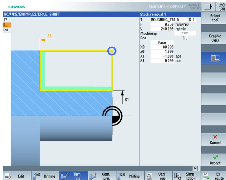
Figure 7-5 Facing the workpiece
