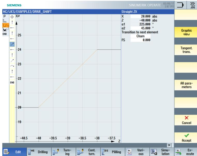
Figure 7-12 Entering the sloping straight-line segment for the contour
