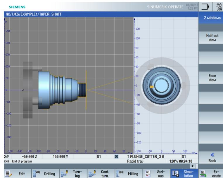
Figure 6-51 Simulation – 2-window view
