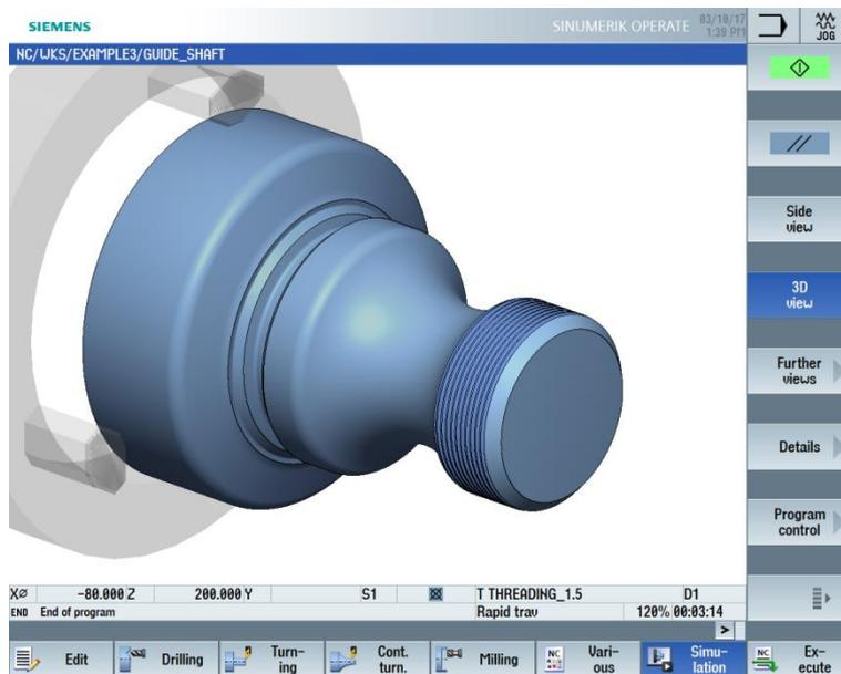
Figure 8-35 Simulation 3D view – Details
