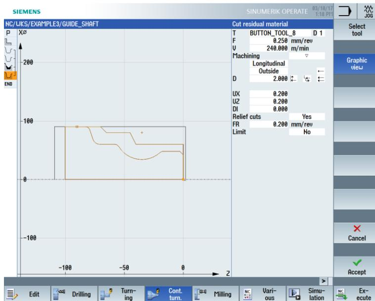
Figure 8-24 Cutting the residual material from the contour
