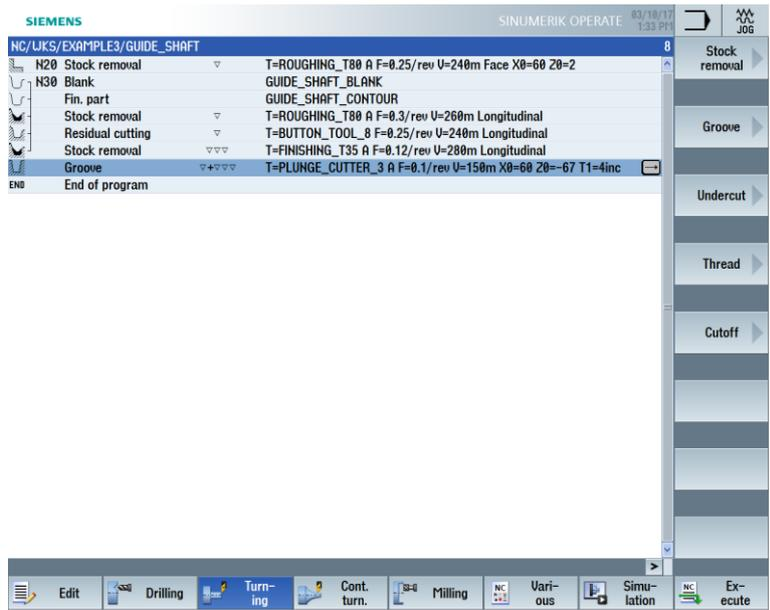
Figure 8-31 Machining plan including groove
