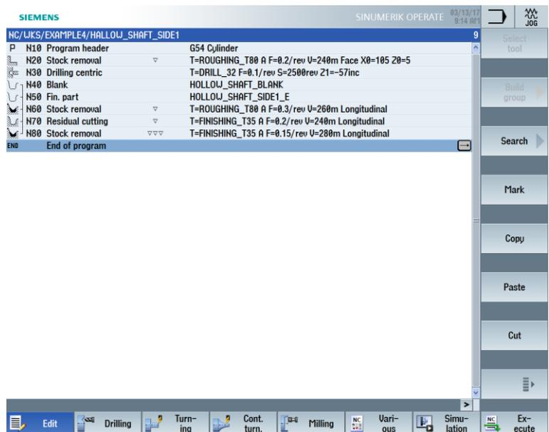
Figure 9-24 Machining plan after machining the contour
