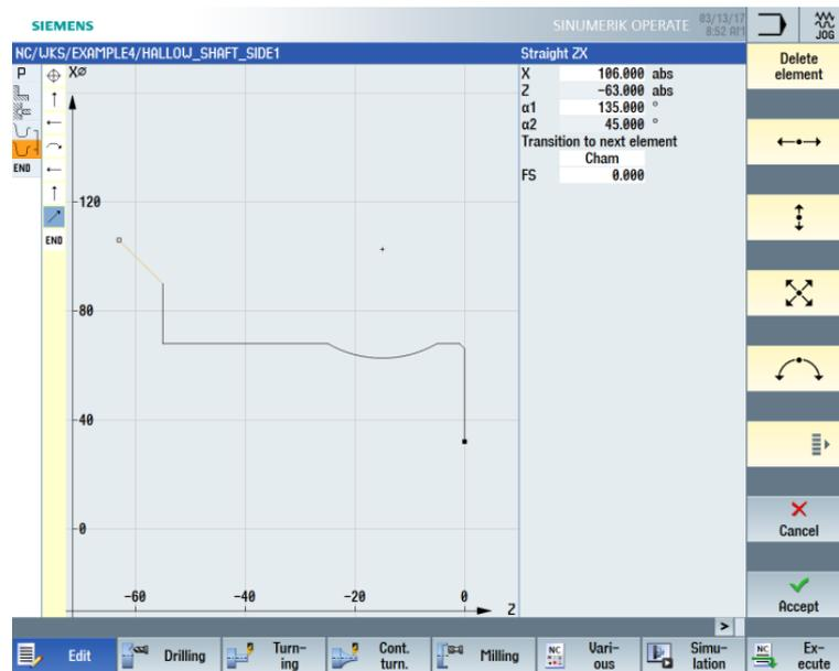
Figure 9-19 Contour in the contour calculator
