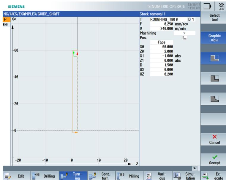
Figure 8-3 Facing the workpiece
