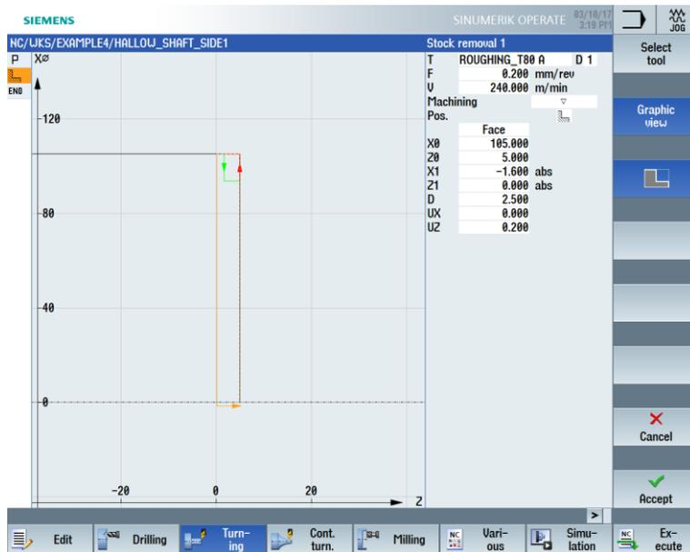
Figure 9-5 Facing the workpiece
