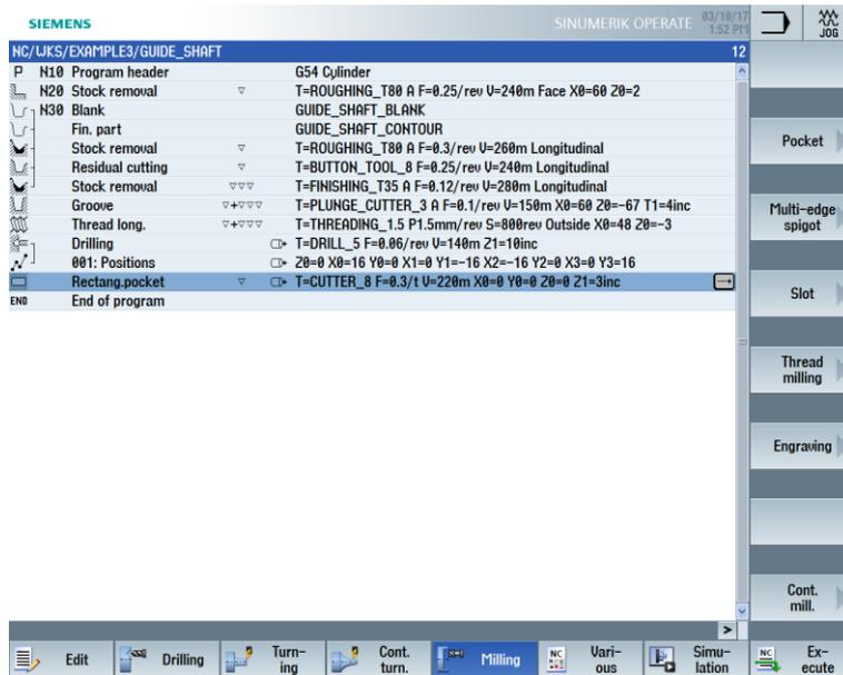
Figure 8-44 Machining plan after rectangular pocket
