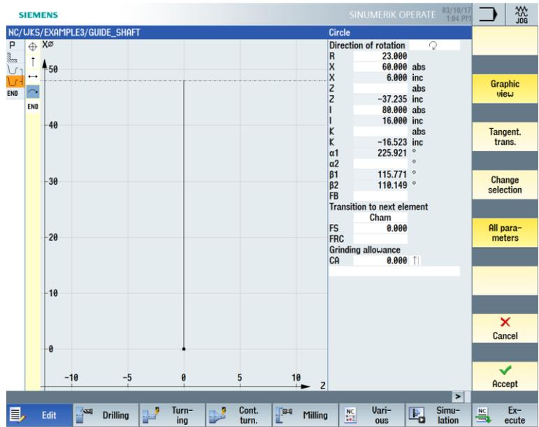
Figure 8-14 Applying the selected arc for the contour
