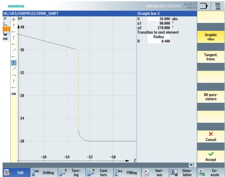
Figure 7-14 Entering the vertical straight-line segment for the contour
