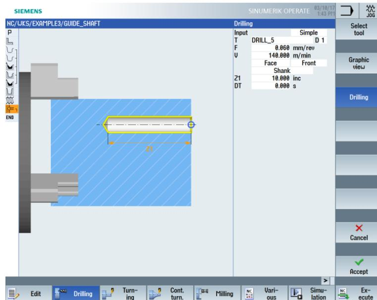
Figure 8-37 Drilling
