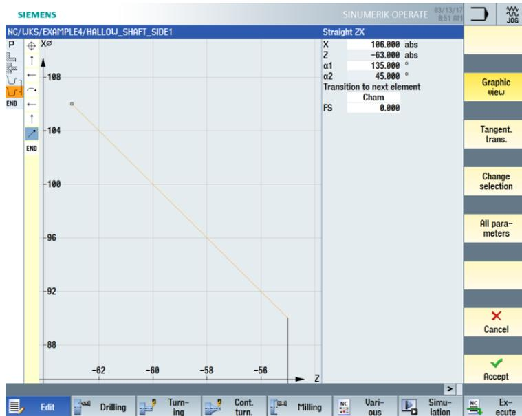
Figure 9-18 Entering the inclined straight-line segment for the contour
