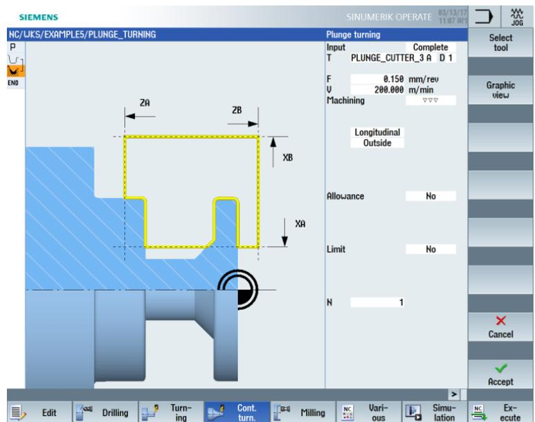
Figure 10-6 Finishing the contour
