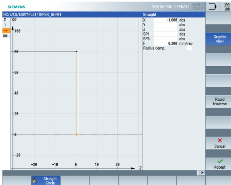
Figure 6-14 Entering the traversing path
