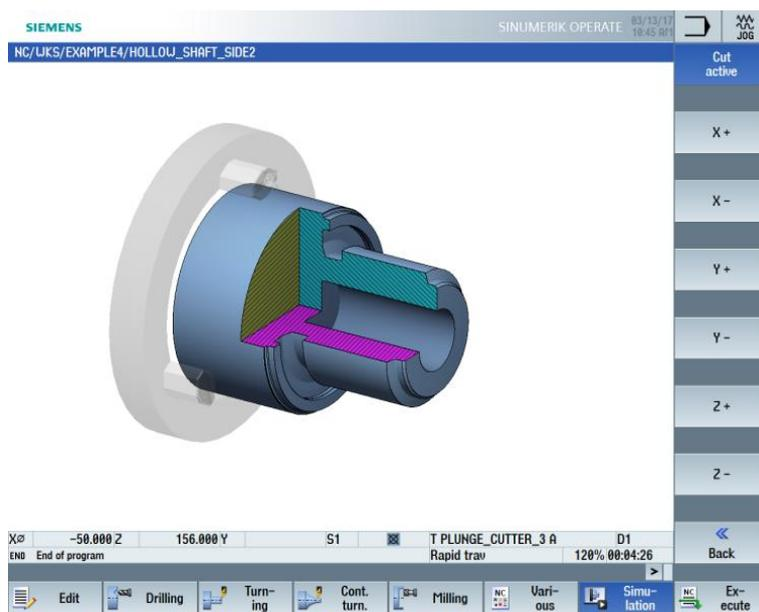
Figure 9-59 Simulation – 3D view (cut active)
