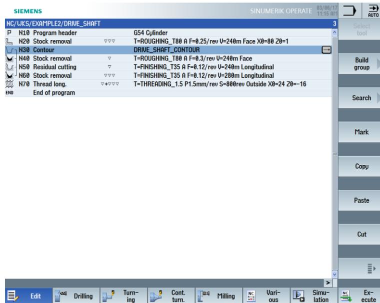
The contour to be machined is entered graphically as a machining step.
