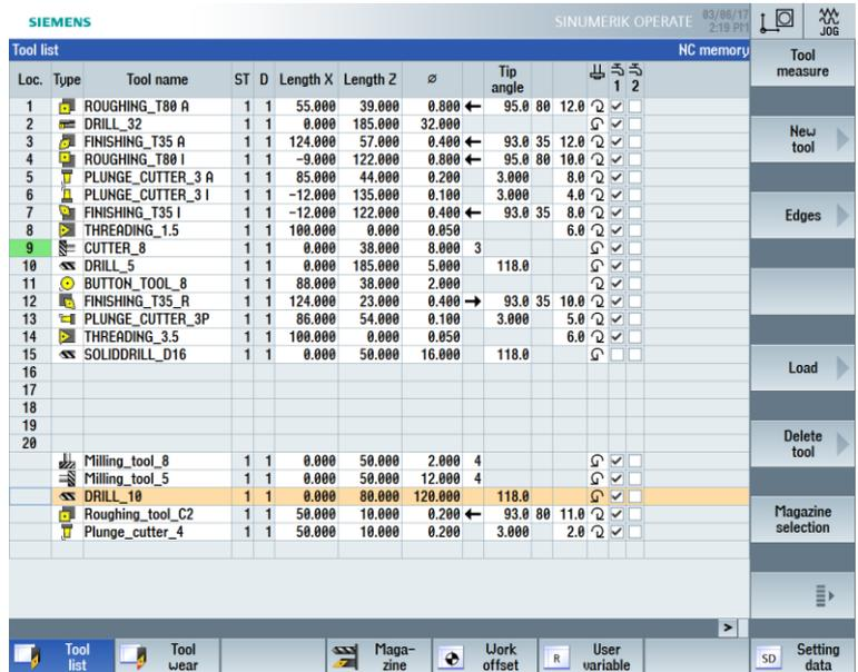
Figure 5-6 Selecting the tool in the magazine
