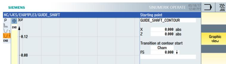
Figure 8-8 Specifying the contour starting point
