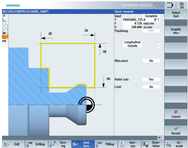
Figure 8-27 Finishing the contour
