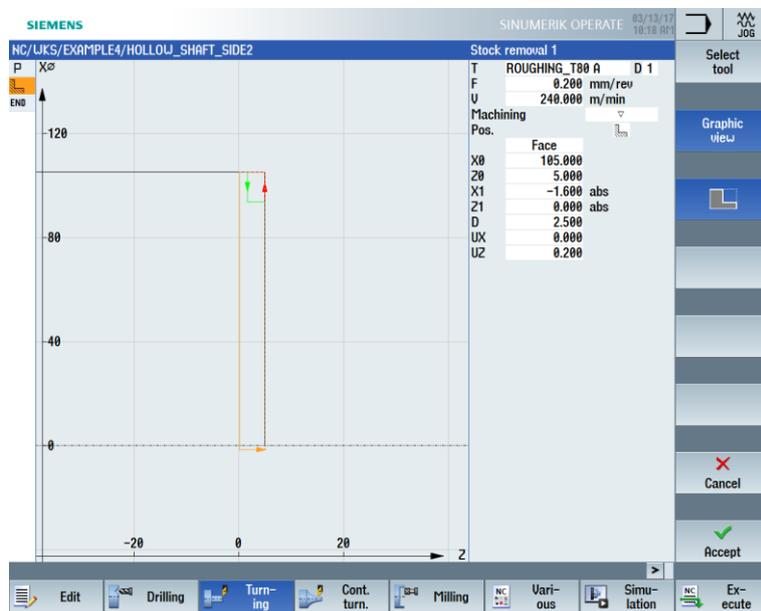
Figure 9-44 Facing the workpiece
