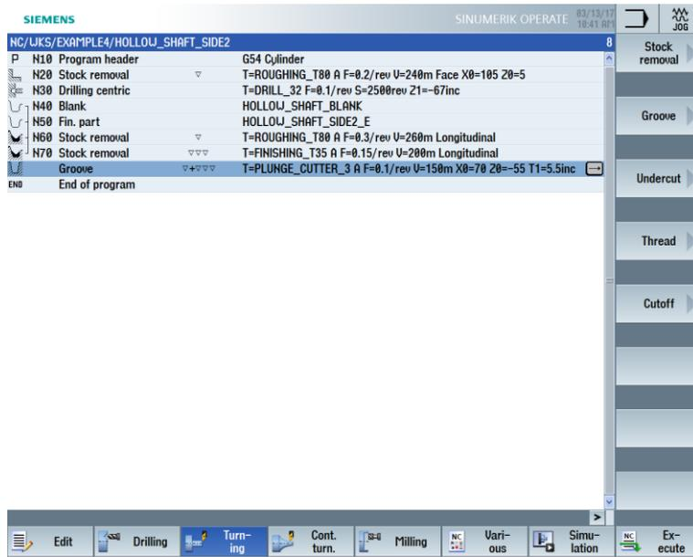
Figure 9-58 Machining plan after groove
