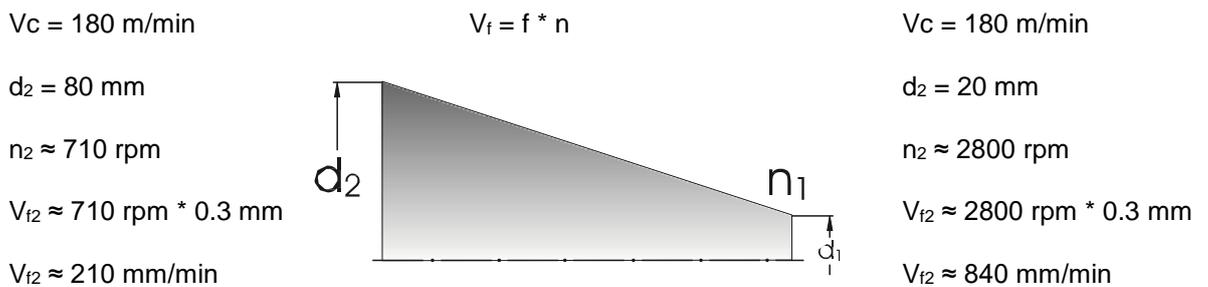
Since the speed is different, the feedrate also differs for the various diameters, despite having the same feed.
