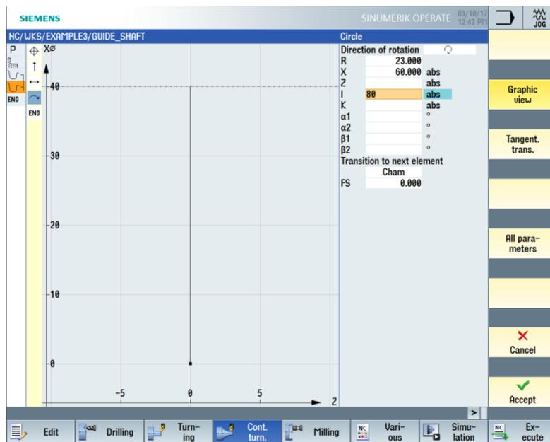
Figure 8-11 Entering the arc for the contour
