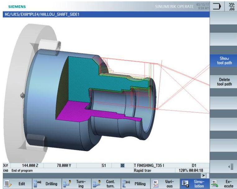
Figure 9-38 Undercut simulation (with display of the traversing paths)
