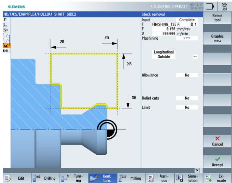
Figure 9-54 Finishing the contour
