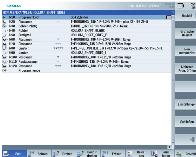
Figure 11-2 Opening the machining plan
