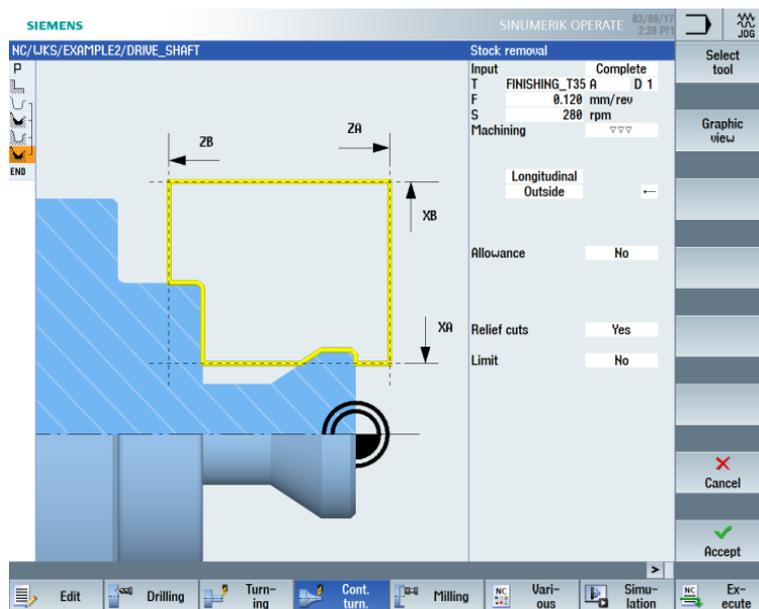
Figure 7-26 Finishing the contour
