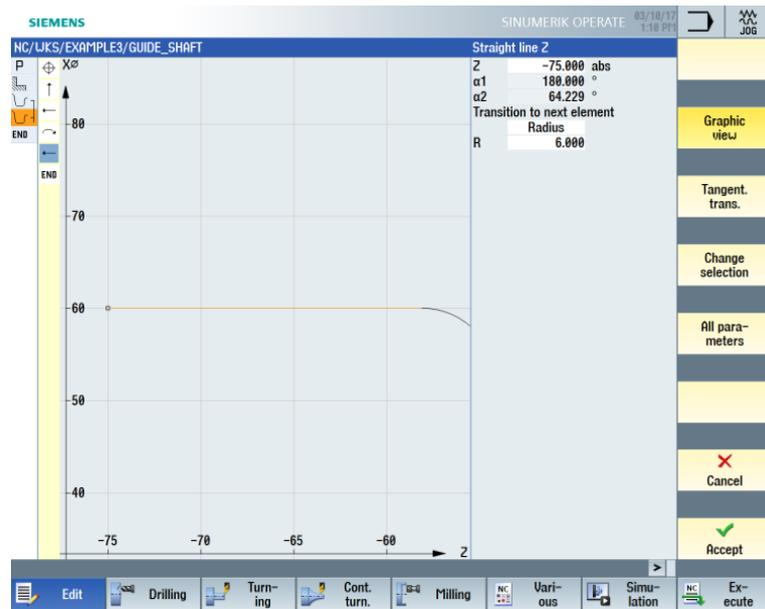
Figure 8-17 Entering the horizontal straight-line segment for the contour
