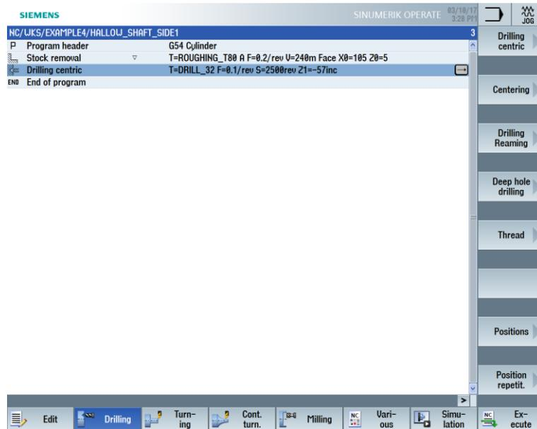
Figure 9-8 Machining plan after drilling
