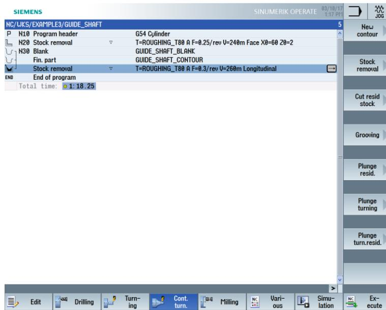
Figure 8-23 Machining plan including roughing machining
