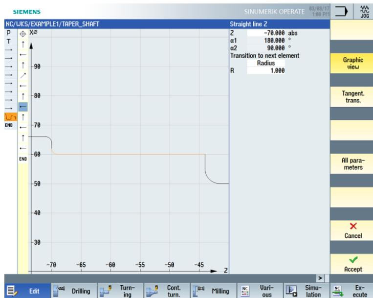
Figure 6-27 Entering the horizontal straight-line segment for the contour
