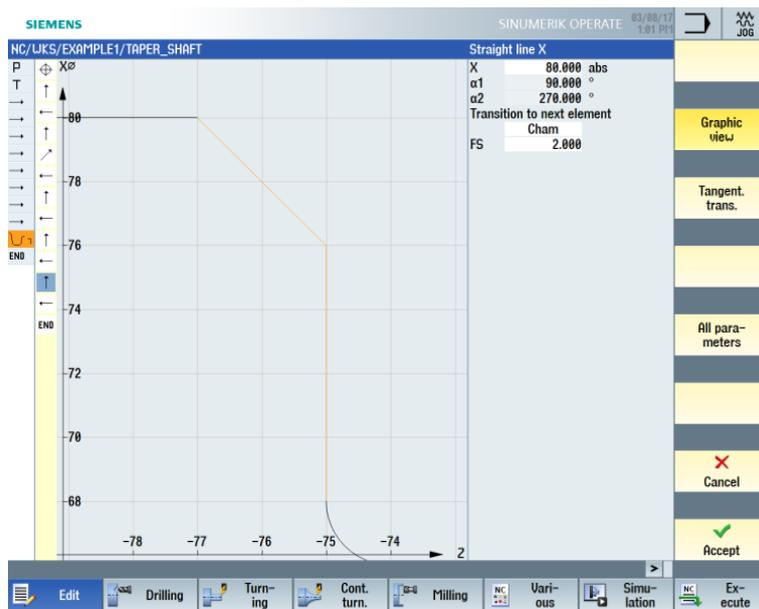
Figure 6-30 Entering the vertical straight-line segment for the contour
