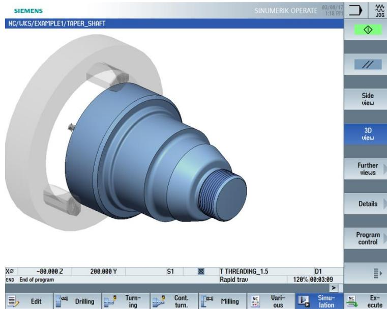
Figure 6-45 Simulation of thread
