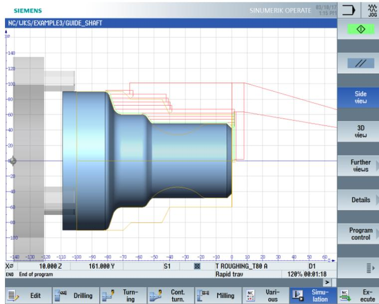
Figure 8-22 Contour stock removal simulation (with display of the traversing paths).
