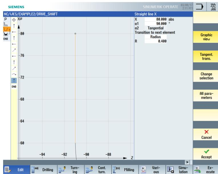
Figure 7-19 Entering the vertical straight-line segment for the contour
