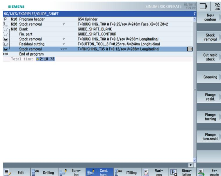
Figure 8-29 Machining plan after stock removal
