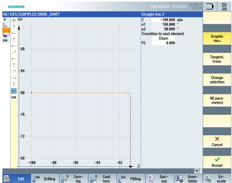
Figure 7-20 Entering the horizontal straight-line segment for the contour
