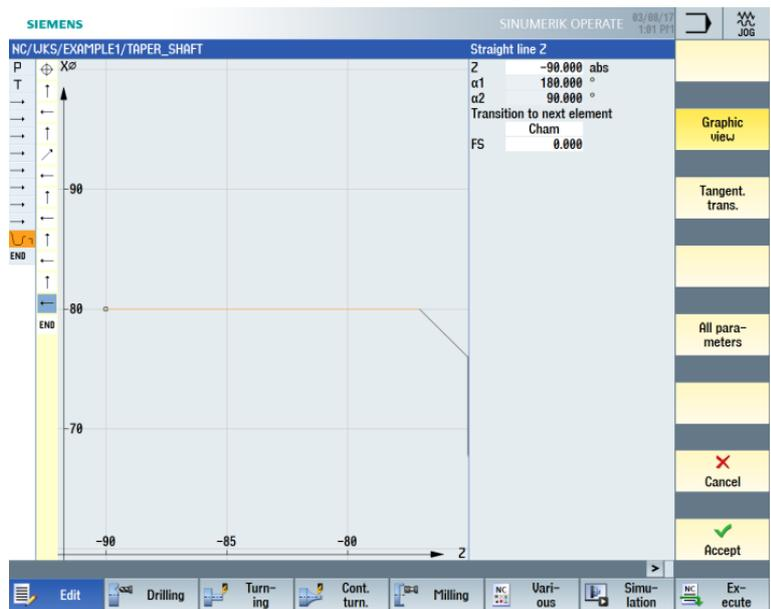
Figure 6-31 Specifying the contour end point
