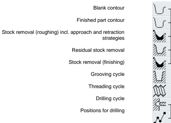
This relationship between geometry and technology is represented very clearly in the graphical display of the machining steps by a "bracketing" of the corresponding symbols. The "bracketing" signifies a linking of geometry and technology to form a machining step.
