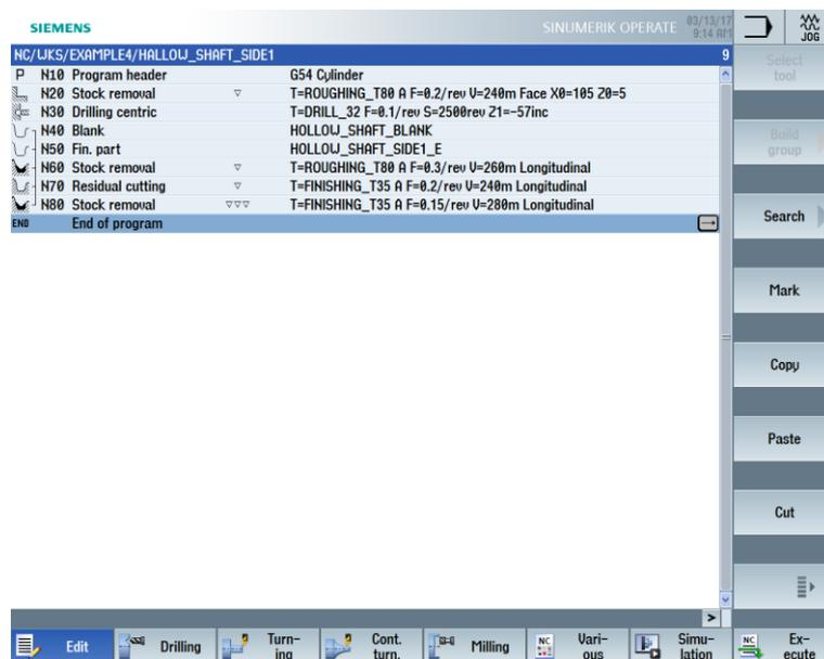
Figure 9-25 Machining plan after stock removal
