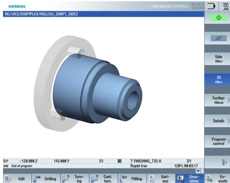
Figure 9-56 Simulation – 3D view
