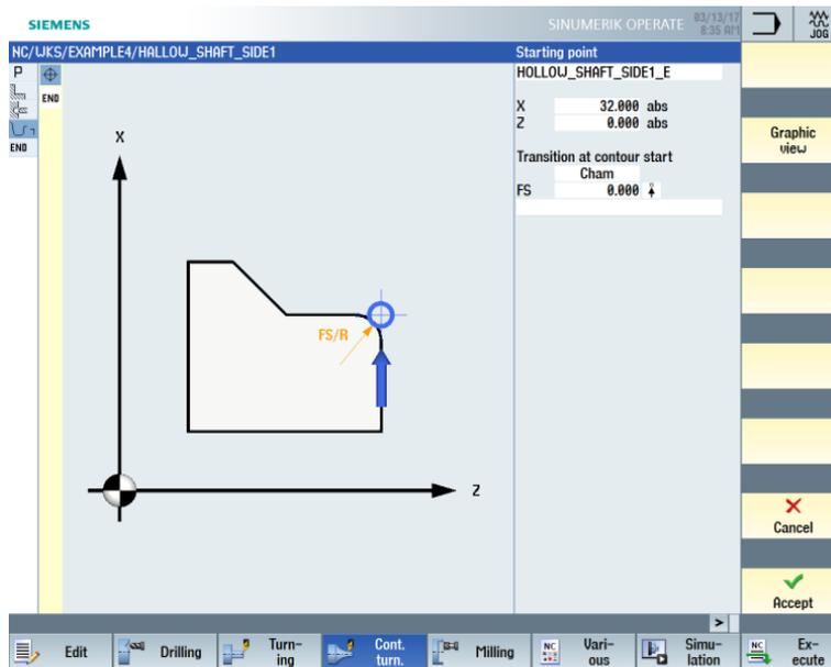
Figure 9-12 Entering the starting point for the contour
