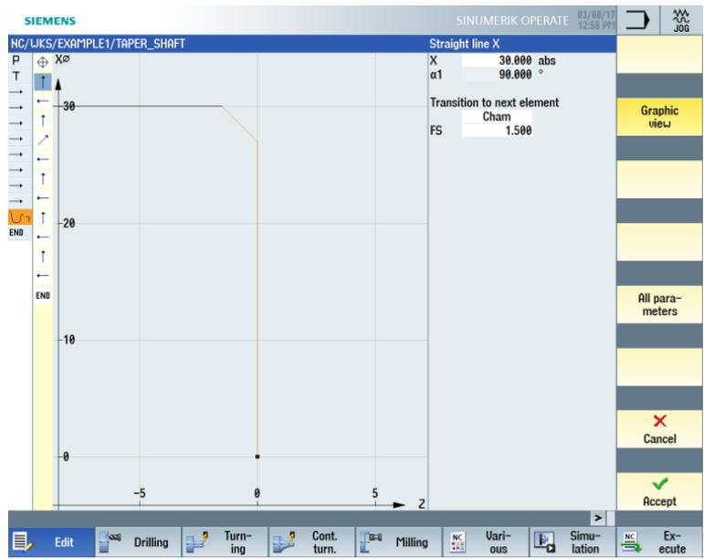
Figure 6-21 Entering the vertical straight-line segment for the contour
