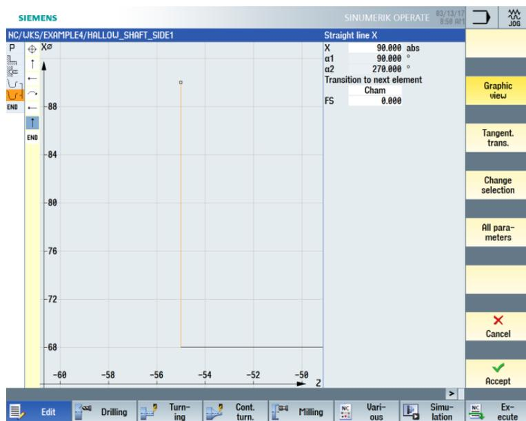
Figure 9-17 Entering the vertical straight-line segment for the contour
