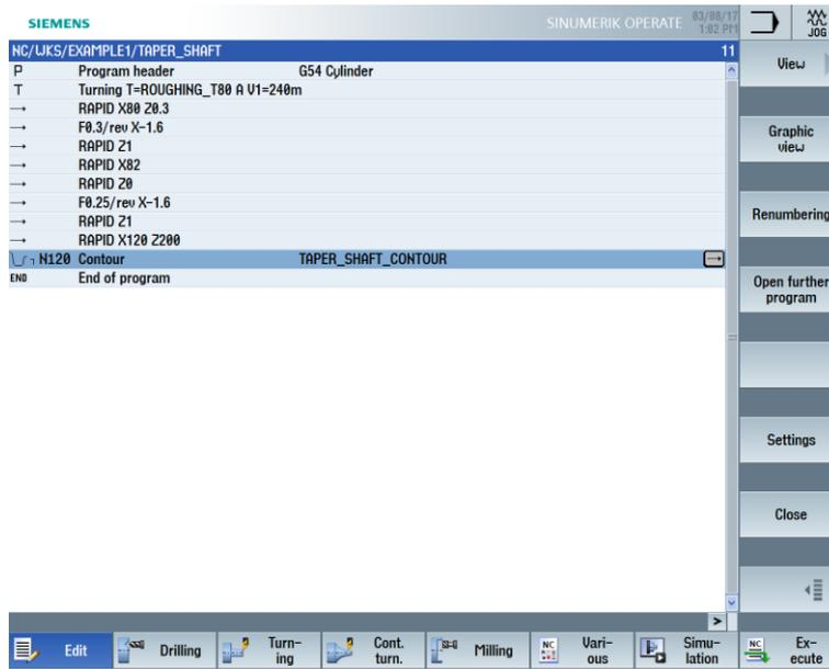
Figure 6-33 Contour in the machining plan
