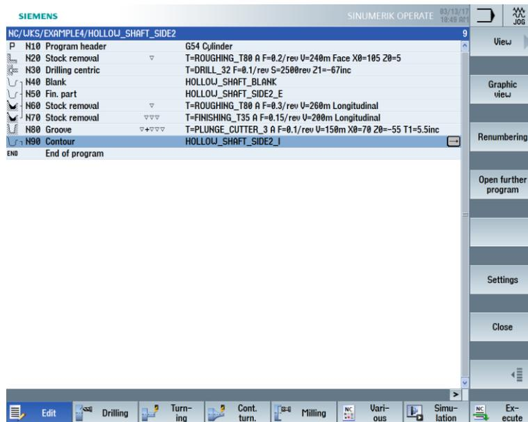
Figure 9-62 Machining plan after input of the contour
