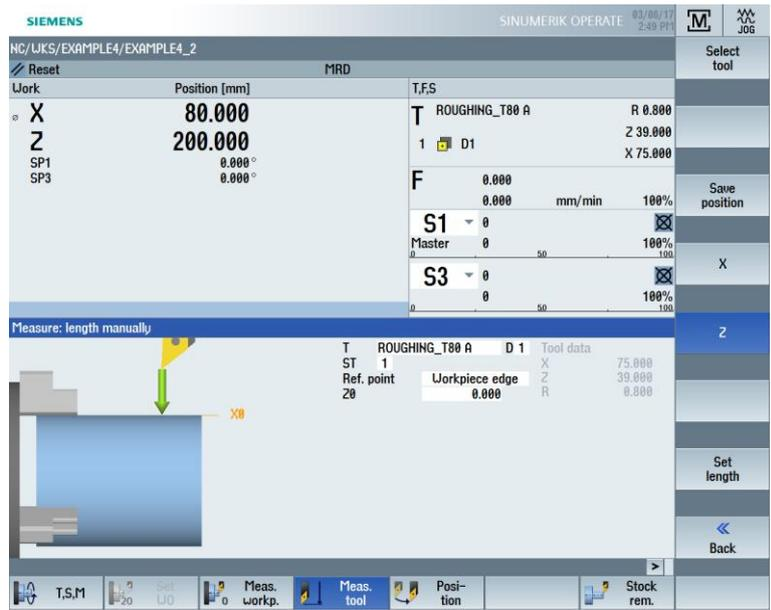
Figure 5-11 Tool measurement – Setting length Z
