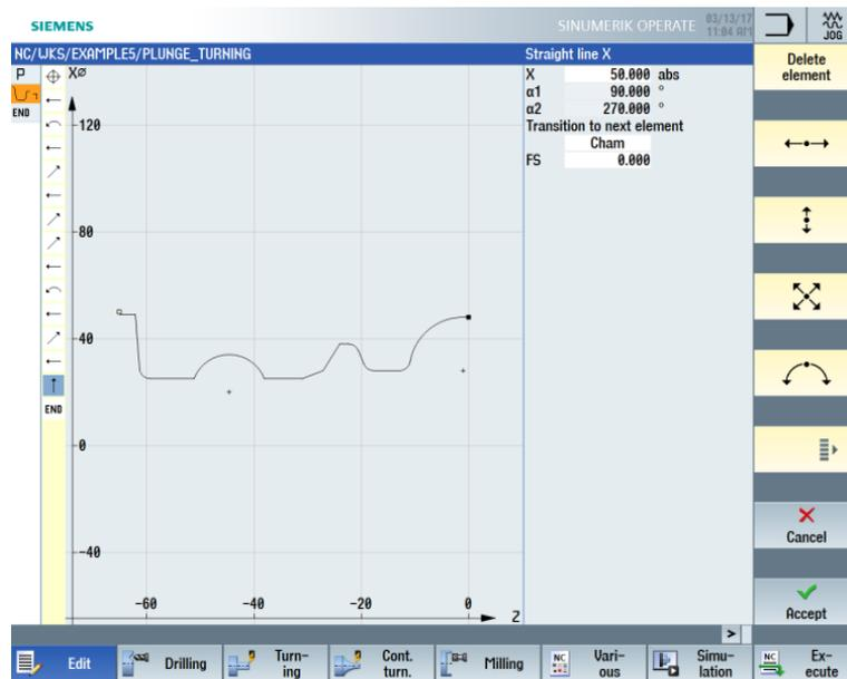
Figure 10-4 Contour in the contour calculator
