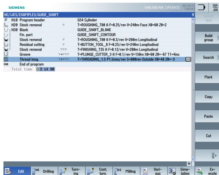
Figure 8-36 Machining plan after thread machining
