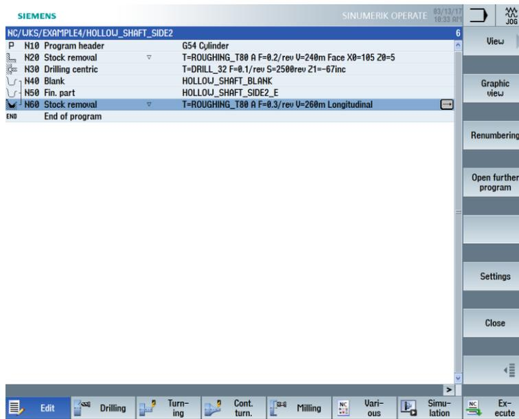
Figure 9-53 Machining plan after roughing
