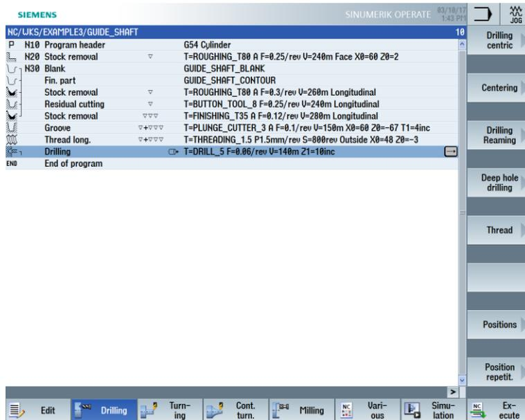
Figure 8-38 Machining plan following drilling
