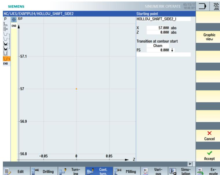
Figure 9-60 Entering the starting point for the contour
