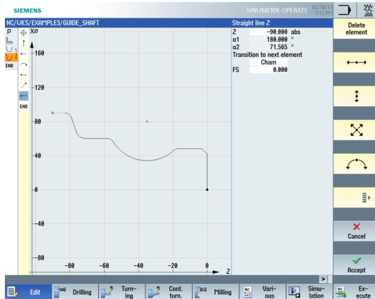
Figure 8-20 Applying the contour
