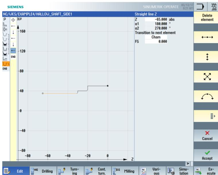
Figure 9-32 Finished part contour of the first side, internal
