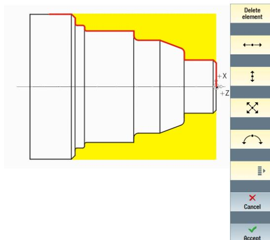
With the graphic contour calculator, you can enter the contours faster and more easily than with conventional programming – and without any math.
