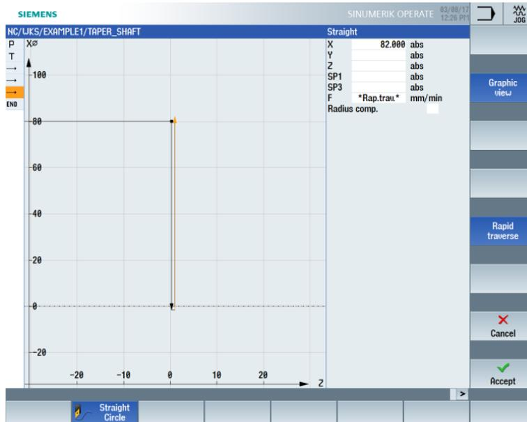
Figure 6-16 Entering the traversing path – Returning to the starting point
