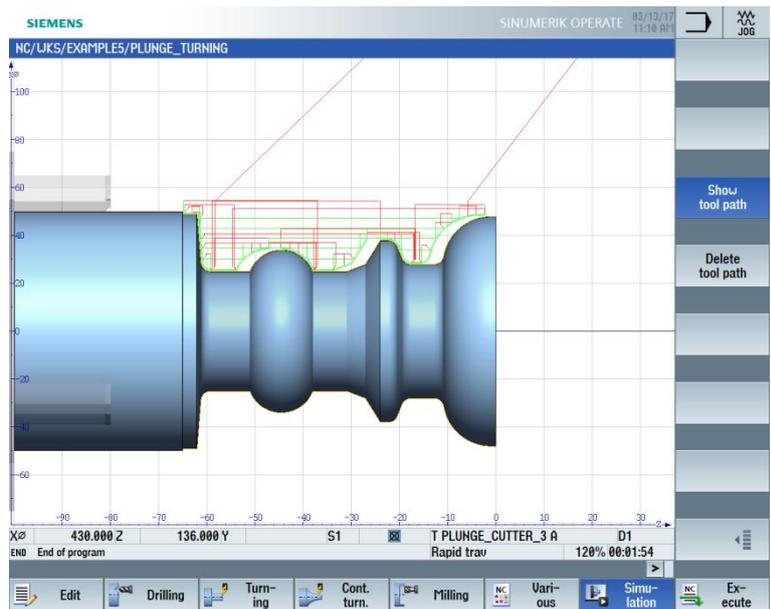
Figure 10-8 Simulation – Side view (with display of the traversing paths)
