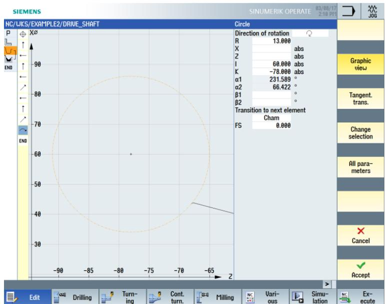
Figure 7-18 Applying the arc for the contour
