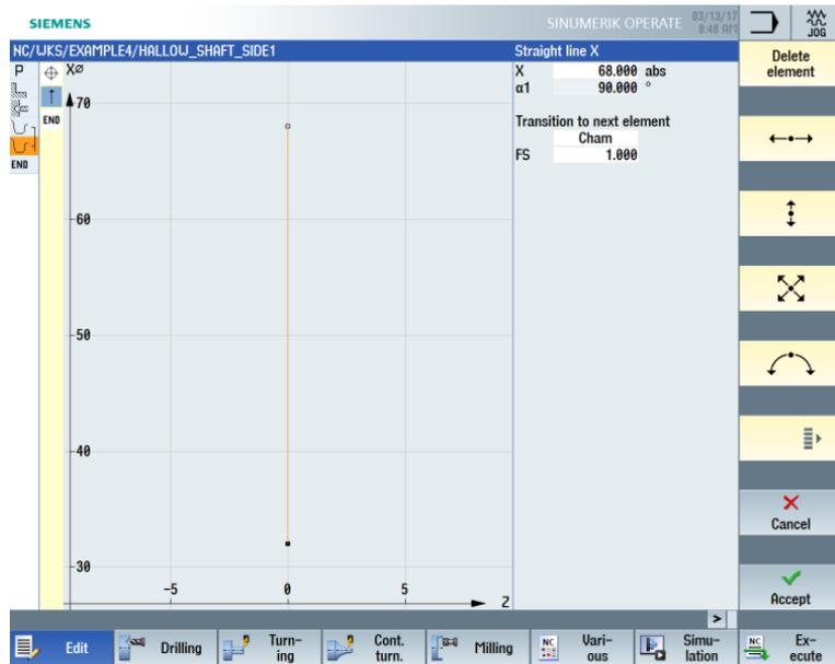
Figure 9-13 Entering the vertical straight-line segment for the contour
