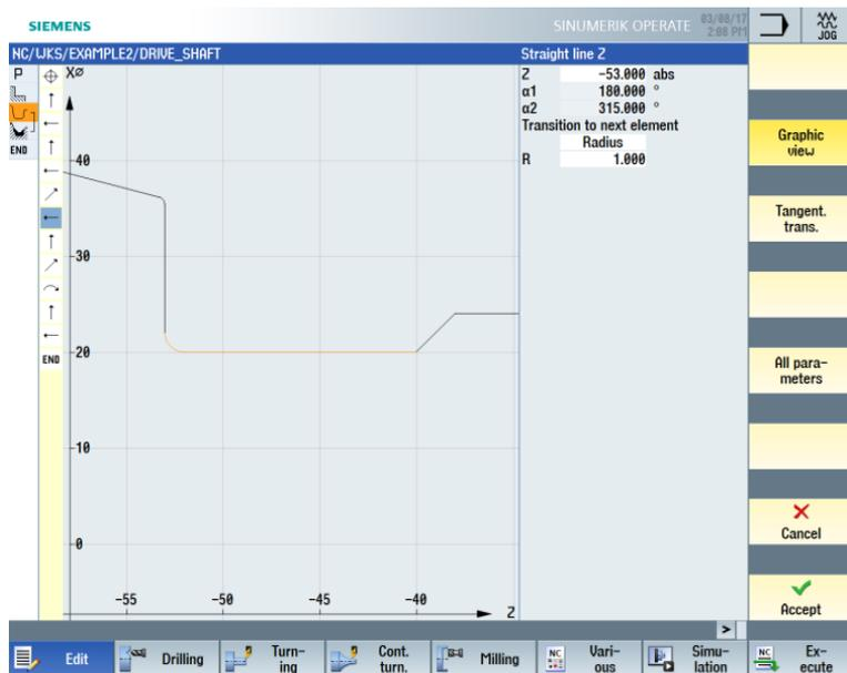
Figure 7-13 Entering the horizontal straight-line segment for the contour
