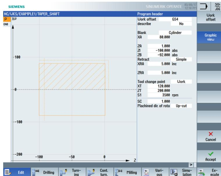
Figure 6-11 Program header – Graphic view
