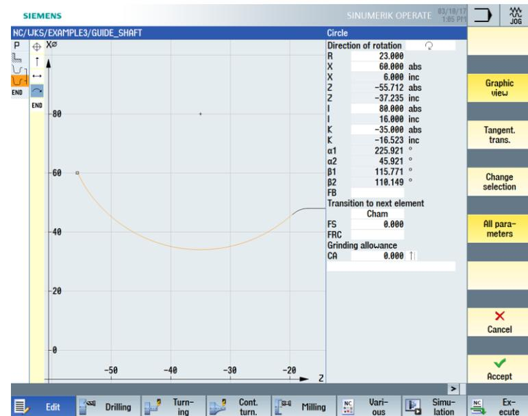
Figure 8-15 Entering the arc center point for the contour
