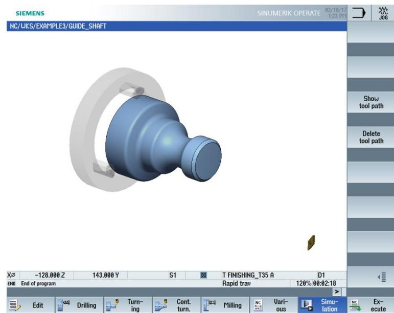
Figure 8-28 Finishing simulation – 3D view
