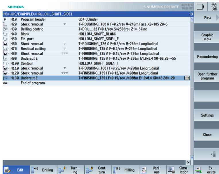
Figure 9-39 Machining plan with undercut
