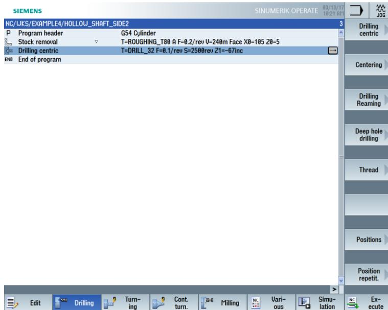
Figure 9-47 Machining plan after input of the drilling position
