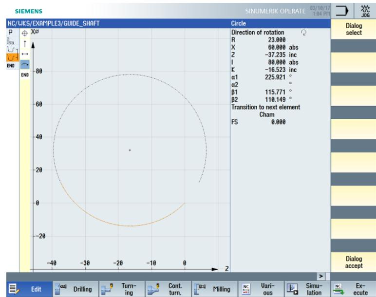
Figure 8-13 Selecting an arc for the contour
