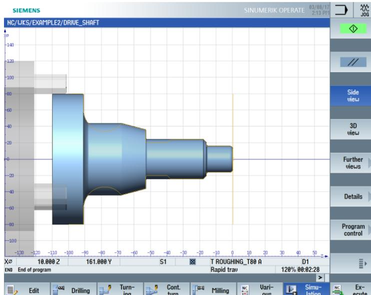
Figure 7-23 Roughing the contour – Simulation side view
