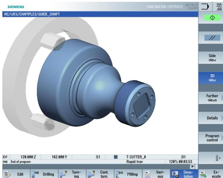
Figure 8-45 Simulation 3D view
