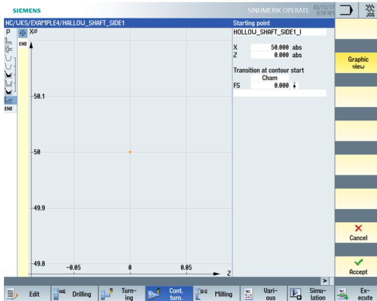
Figure 9-31 Entering the starting point for the contour
