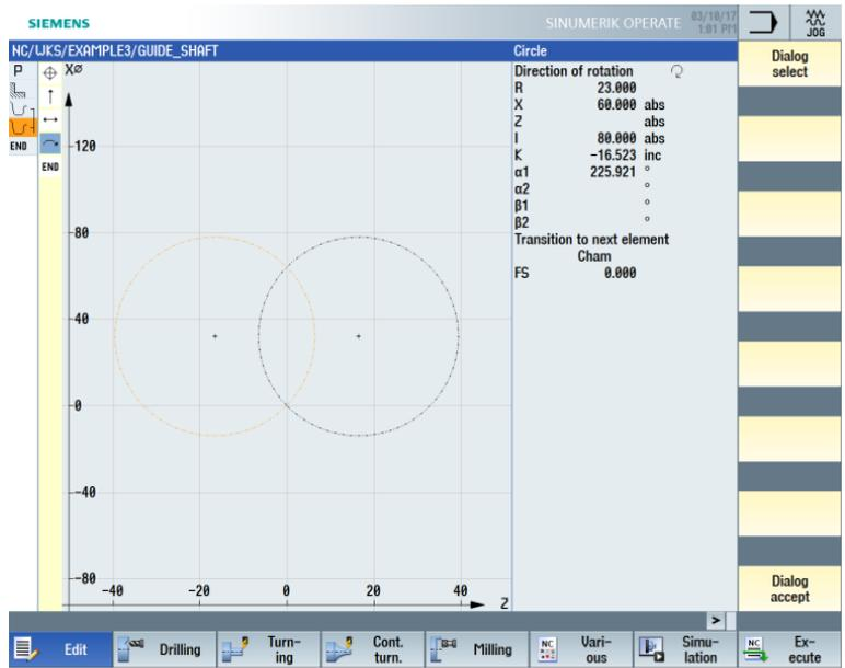
Figure 8-12 Selecting an arc for the contour
