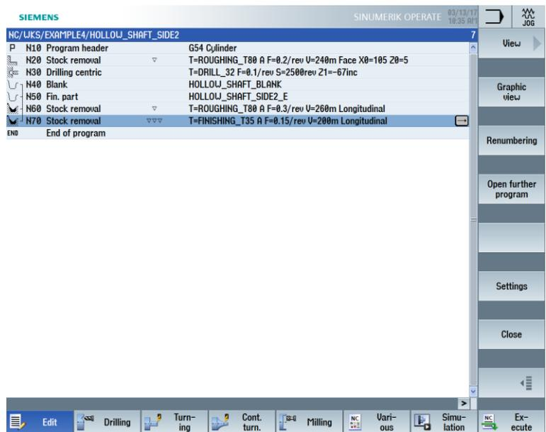
Figure 9-55 Machining plan after machining the contour
