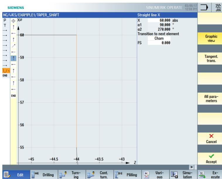
Figure 6-26 Entering the vertical straight-line segment for the contour
