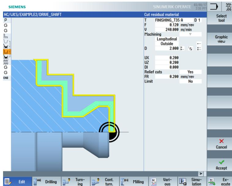
Figure 7-24 Contour: Cutting the residual material
