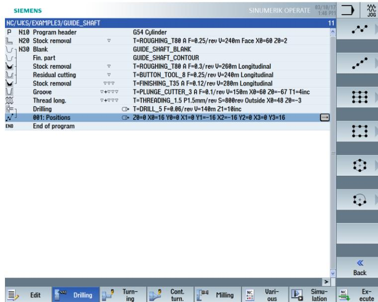
Figure 8-40 Machining plan after input of the position pattern
