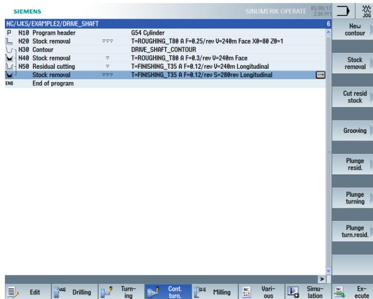
Figure 7-27 Machining plan
