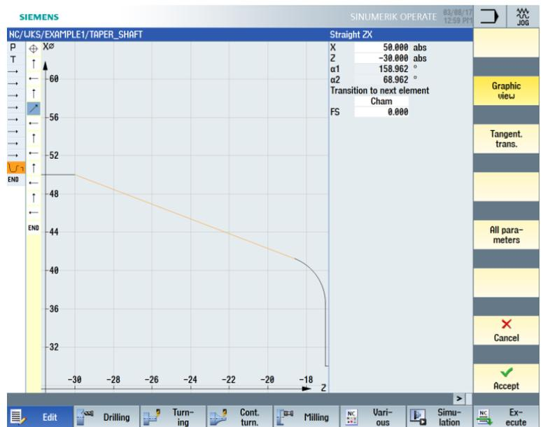
Figure 6-24 Entering the end point of the inclined straight line for the contour
