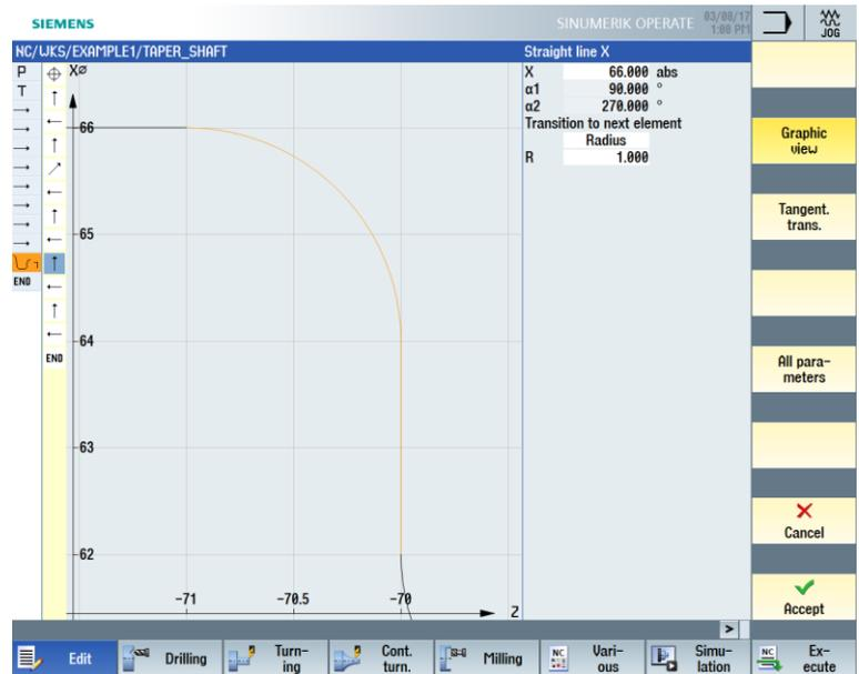
Figure 6-28 Entering the vertical straight-line segment for the contour
