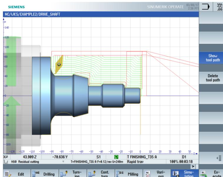
Figure 7-25 Cutting residual material – Simulation side view
