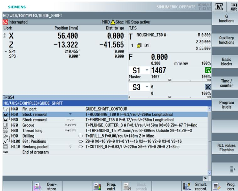
Figure 3-3 Executing the machining plan
