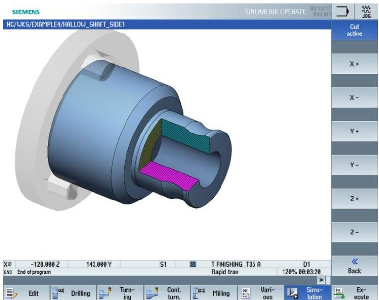
Figure 9-28 Simulation – Cut active
