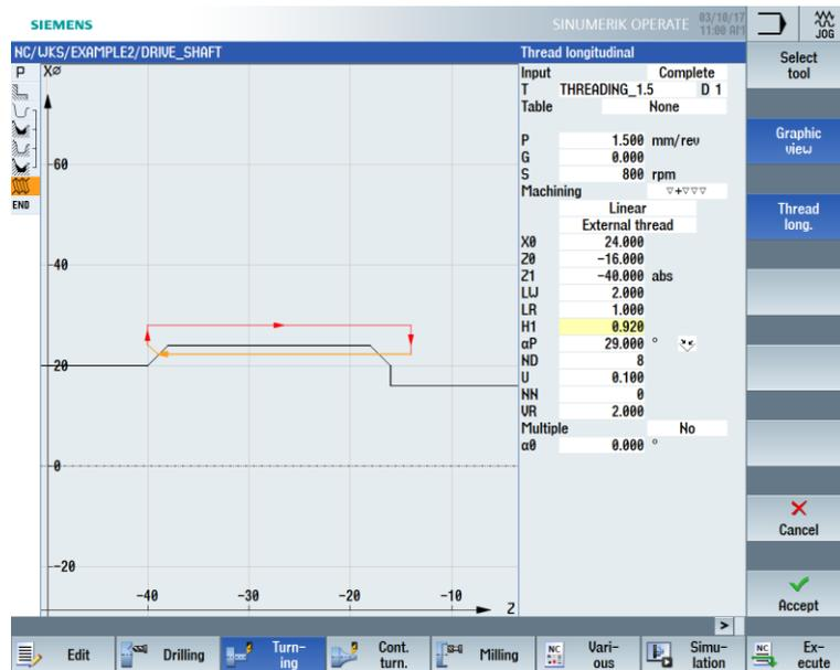
Figure 7-29 Producing the thread
