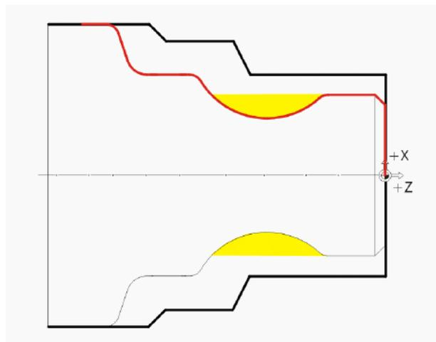
The following figure shows the machining plan up to and including the roughing machining:
