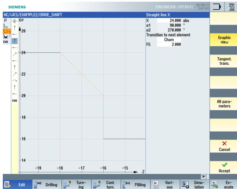
Figure 7-10 Entering the vertical straight-line segment for the contour
