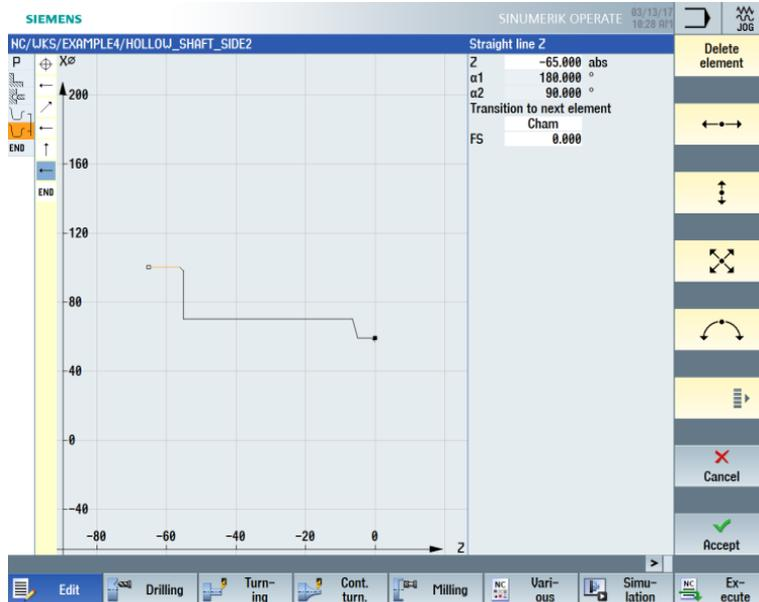
Figure 9-51 Contour in the contour calculator
