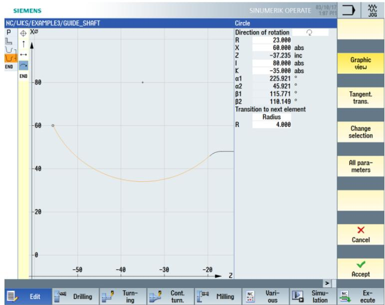
Figure 8-16 Entering the arc radius for the contour
