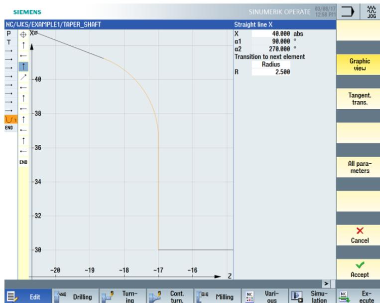
Figure 6-23 Entering the vertical straight-line segment for the contour
