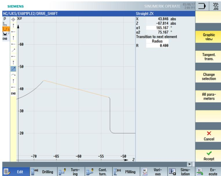
Figure 7-15 Entering the inclined straight line for the contour
