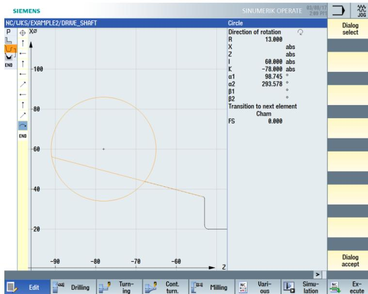
Figure 7-16 Entering the arc for the contour
