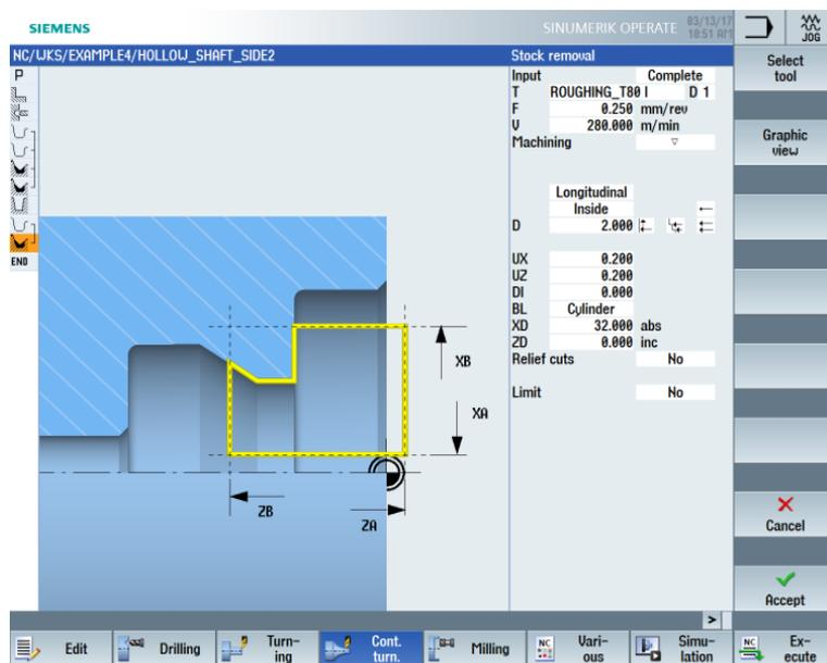
Figure 9-64 Residual stock removal from contour
