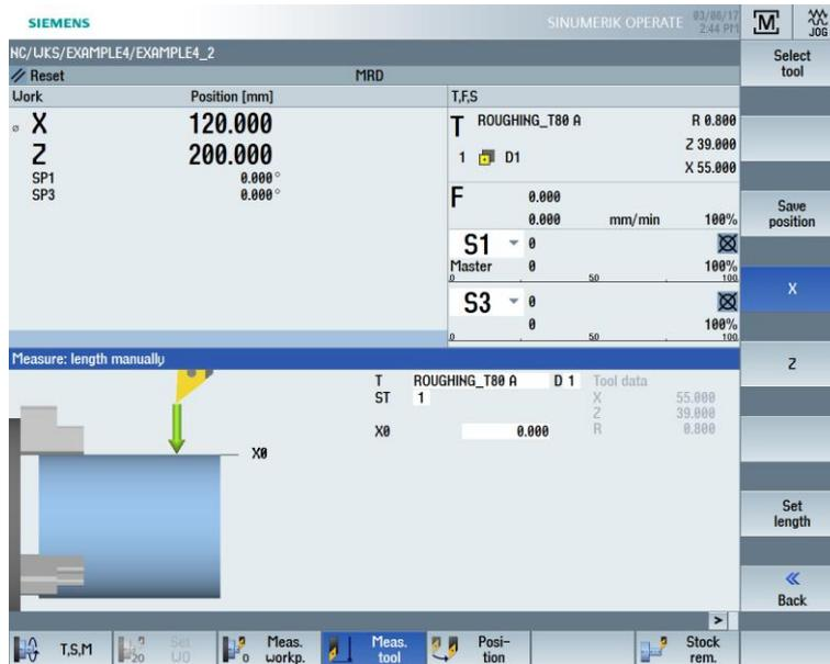
Figure 5-9 Tool measurement – Specification of the X value
