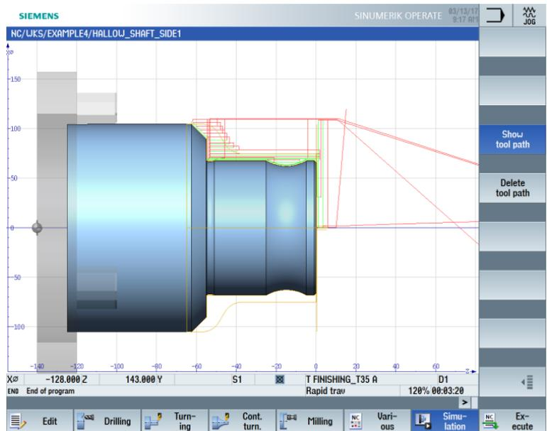
Figure 9-29 Simulation – Side view with display of the traversing paths
