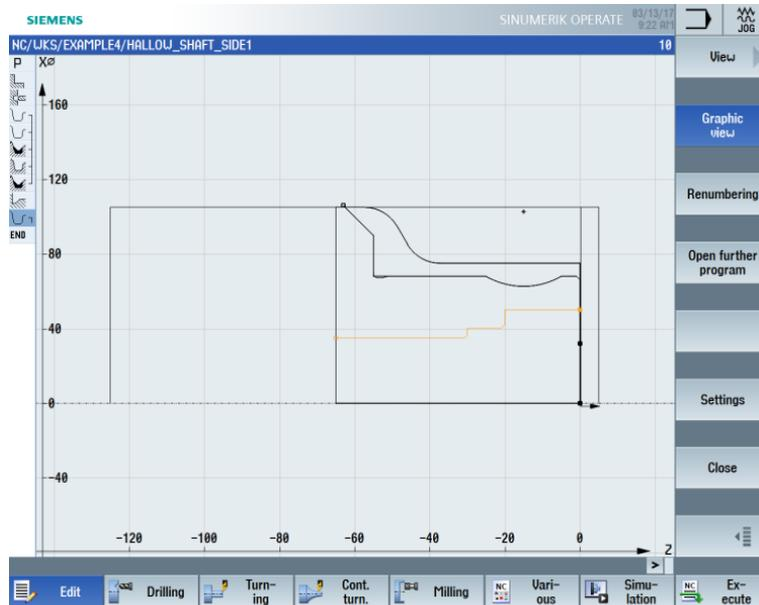
Figure 9-33 Broken-line graphic
