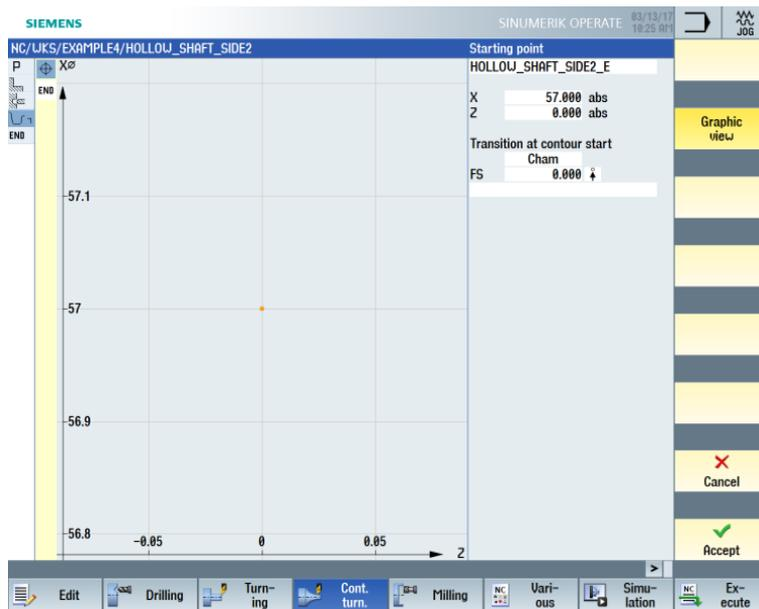
Figure 9-50 Entering the starting point for the contour
