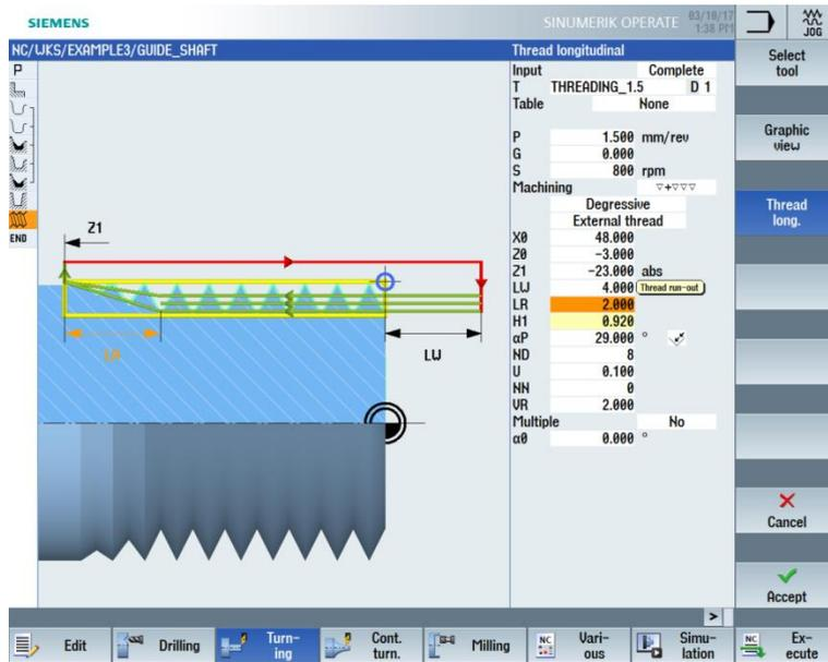
Figure 8-34 Help screen - thread run-out
