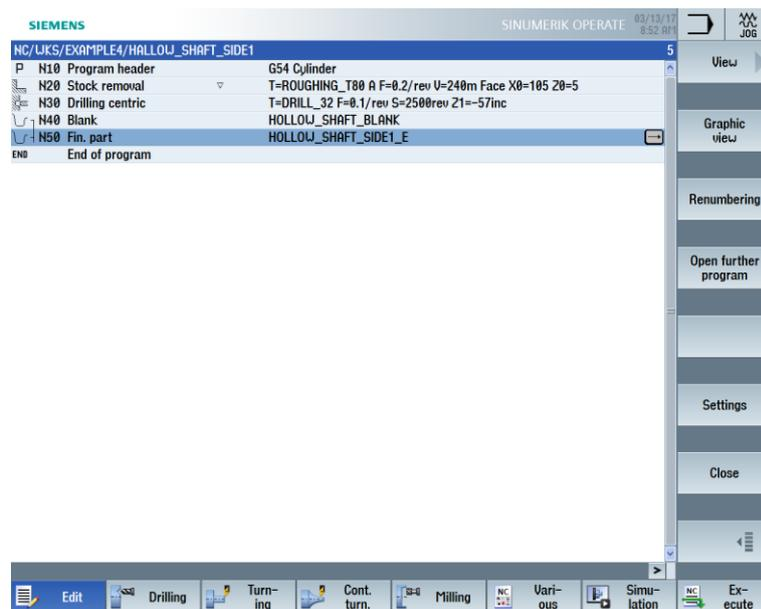
Figure 9-20 Machining plan after input of the contours
