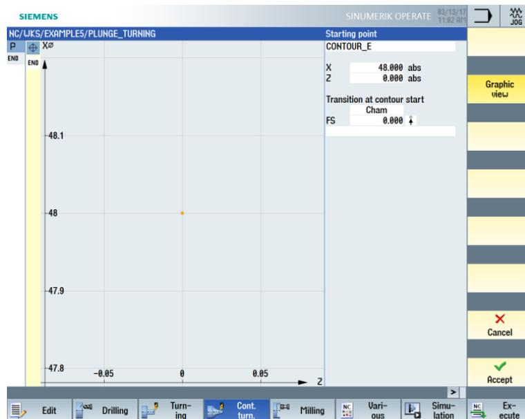
Figure 10-3 Entering the starting point for the contour
