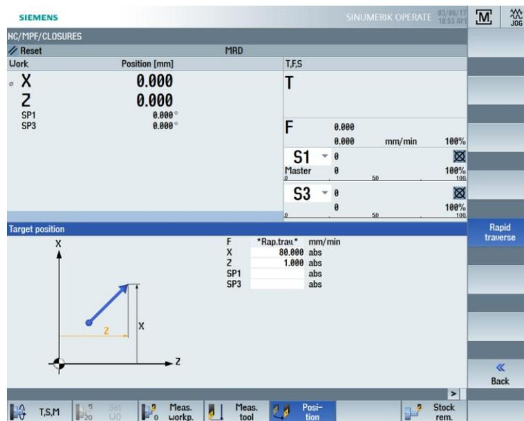
Figure 3-2 Specification of a target position
