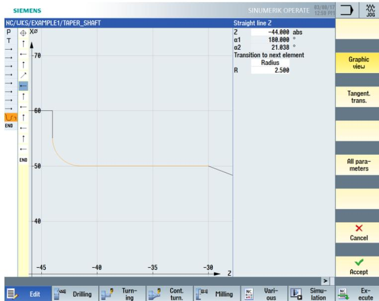
Figure 6-25 Entering the horizontal straight-line segment for the contour
