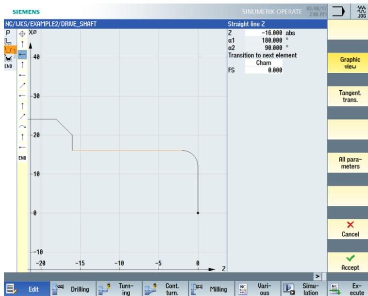
Figure 7-9 Entering the horizontal straight-line segment for the contour
