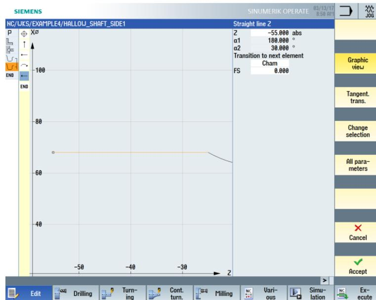
Figure 9-16 Entering the horizontal straight-line segment for the contour
