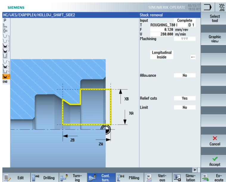
Figure 9-65 Finishing the contour
