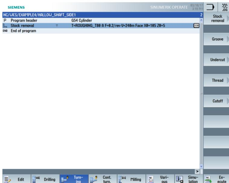
Figure 9-6 Machining plan after face turning
