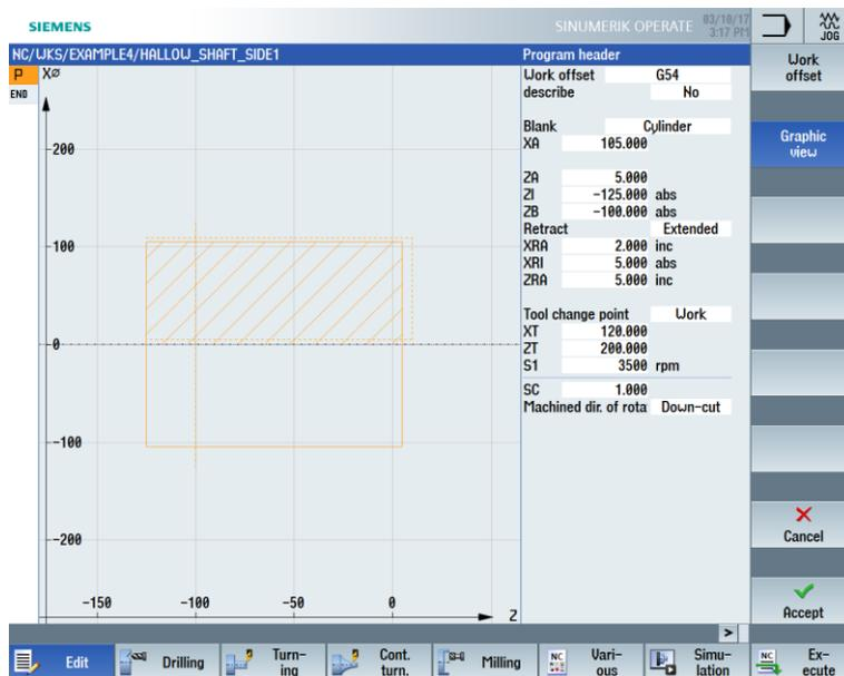
Figure 9-4 Workpiece dimensions in the program header
