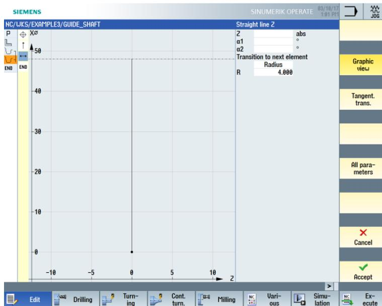
Figure 8-10 Entering the horizontal straight-line segment for the contour
