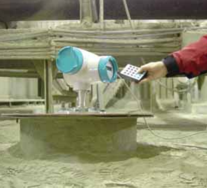
Configuration of the SITRANS LR460 can be performed with a non-intrusive infrared handheld programmer.
