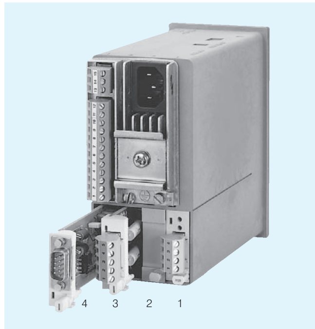
Fig. 5/2 SIPART DR21 controller - rear view, slots
