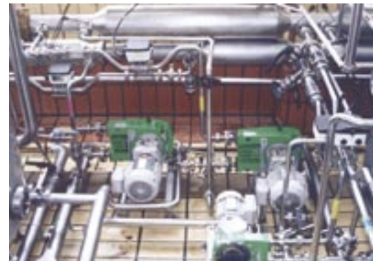
Part of the filtration plant with MAGFLO sensors installed, measuring antioxidant and foam stabilizer.
