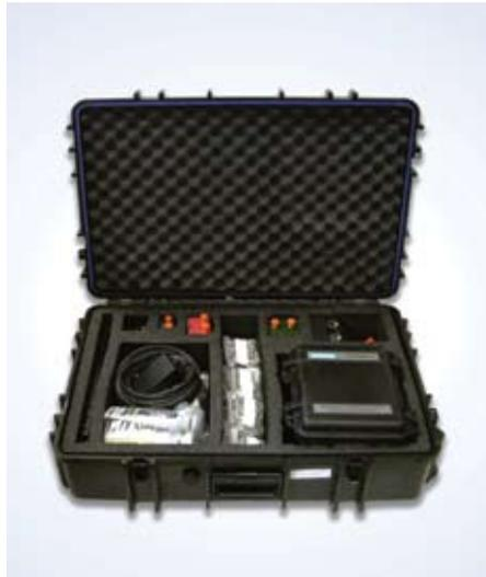
■ Figure 2. The Sitrans FUP1010 check-metering kit from Siemens is delivered with all the tools necessary to perform flowmeter verification
