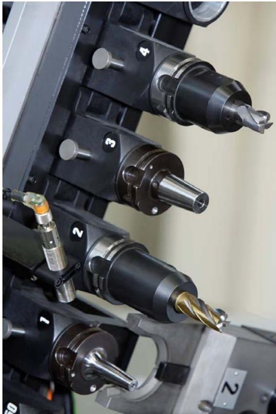
The sonar proximity switch checks whether the place in the tool changer is really free before reinserting the tool
