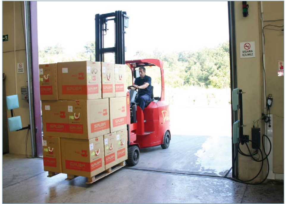
The RFID antennas on the warehouse doors ensure automatic recording of incoming and outgoing goods.
