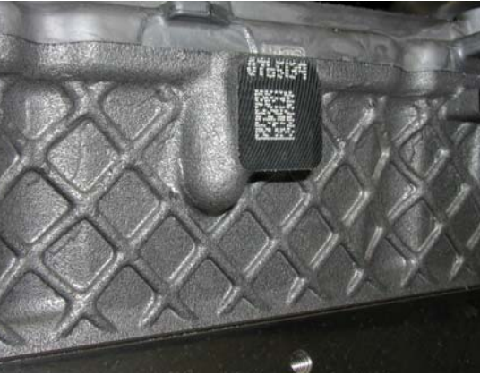
Well-founded quality: A dot-peened Data Matrix code enables the unique identification and traceability of all cylinder heads installed at Daimler MCG / Powertrain.
