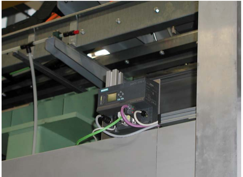
Built-in intelligence: The analysis unit of the VS130-2 analyzes the camera images and sends the result over PROFIBUS DP to the process control level in the form of a data string.
