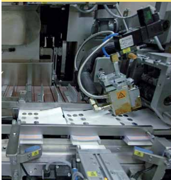
The packaging machine allows fully automatic folding, bonding, and filling of the packaging
