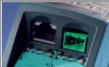
For good connections: Electrical and LAN connection on power insert
