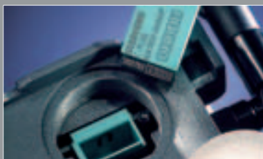
For fast start after unit replacement: C-PLUG stores device data
