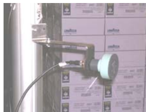
Picture 2: SLA81 read/write antenna for reading and acquiring data stored on the transponders
