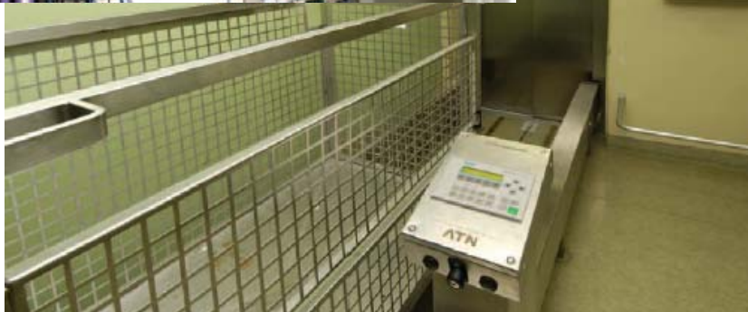
Integrated controller and operator panel: The complete control system Simatic C7-621 accomplishes all tasks required by a 2-space magazine.
