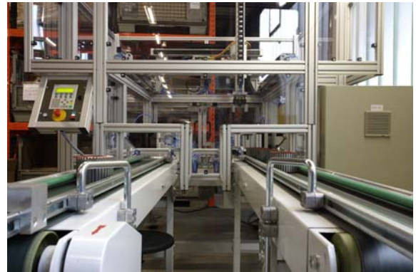
Progress at a six times faster pace: The conveyor belt on the right is the materials buffer of the paper insulating machine; on the left, the insulated stators are transported away
