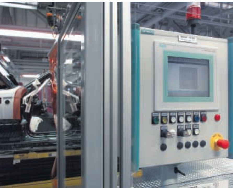
The locally mounted manual HMI device with Simatic MP 270B for distributed HMI and emergency stop function
