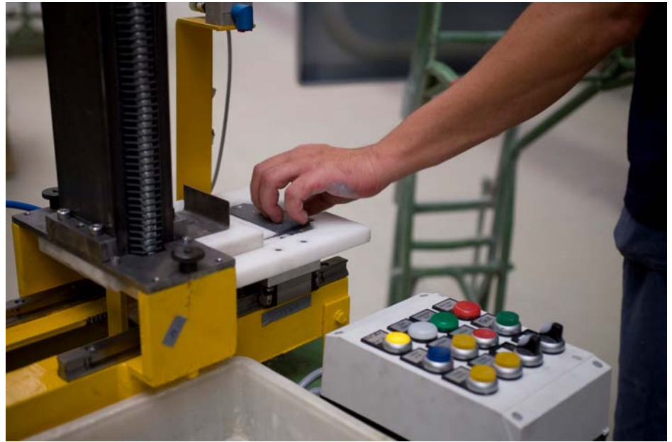
During the firing of the enameled coating, the data is carried along by software. Afterwards, each tub/tray or shower floor receives a new tag – pictured is the manual write station.
