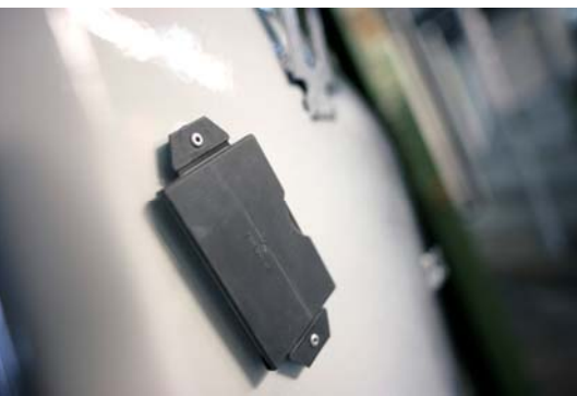
A magnet provides for the safe hold of the credit-card-sized data media RF360T on the product.
