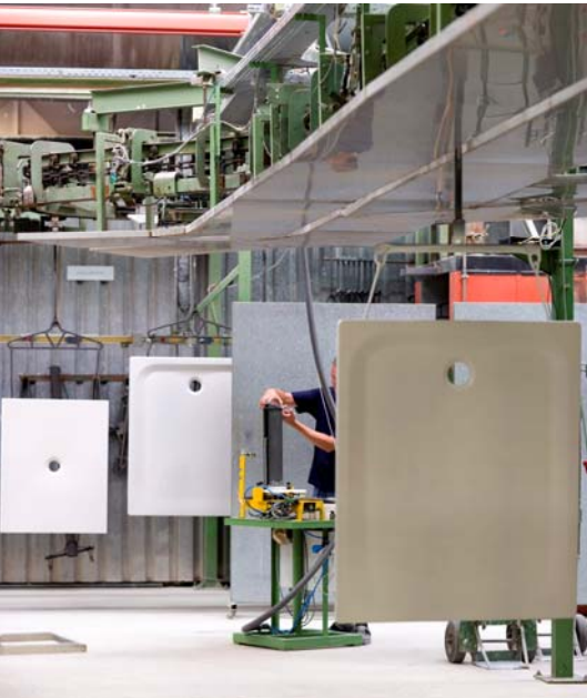
All processing steps are customer-specifically assigned and product-specifically acquired via the RFID system RF300.
