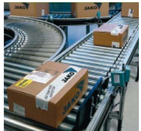
Picture 2: The packages are detected by a photo sensor
