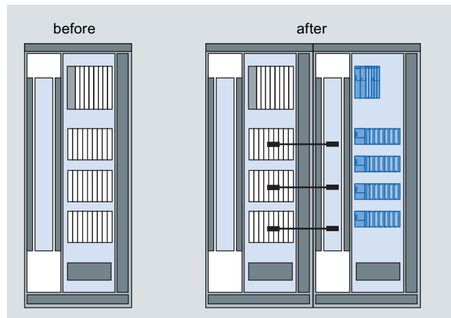
Replacement of TELEPERM M I/O modules by ET 200, version 2
