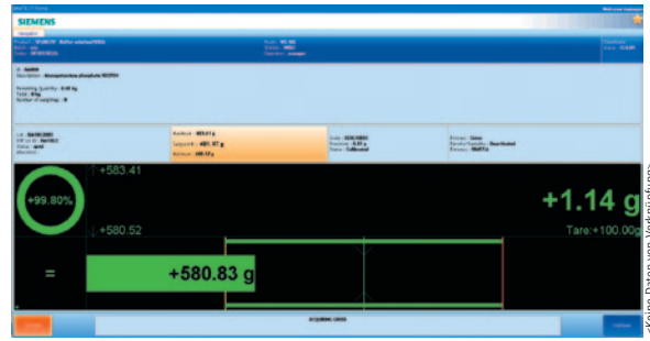
The Simatic IT library for Life Sciences offers compliance-ready modules for typical life science applications such as weighing and dispensing
