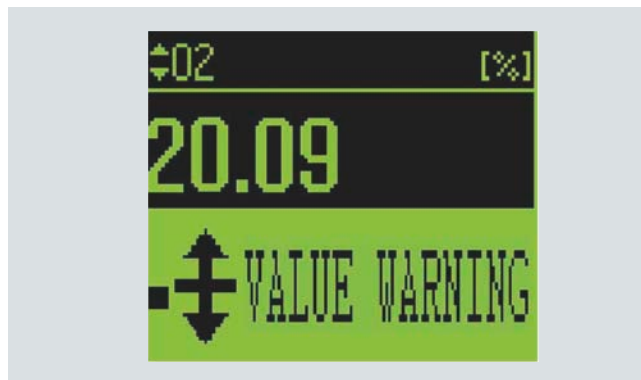
Local user interface (LUI) of SITRANS SL in the detector unit (display of measured value)
