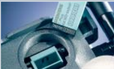
For a quick start after device replacement: C-Plug stores device data
