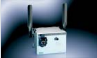
Two antennas for diversity: Reliable transmission and reception
